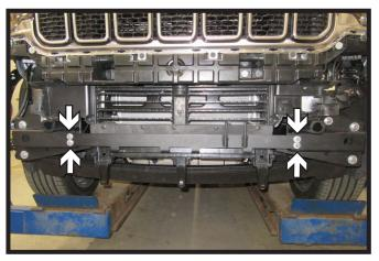
10. Attach cross member to baseplates, start four (4) 3/8" x 1" bolts with flat washers and nylon lock washers. Ensure baseplate is level and tighten baseplate on each side then cross member.
