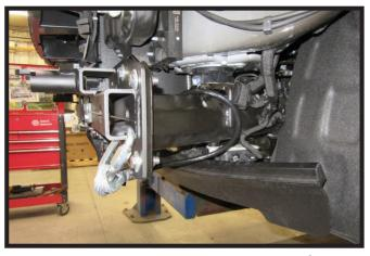
16. Attach the permanent baseplate safety cables to the provided convenience link on the baseplate. The photo above shows the recommended installation of the cables to frame of vehicle. Additional options may interfere with suggested mounting; in this case, secure the cables to a solid piece of the frame as described in the General Information sheet. Be sure the safety cables do not rub against any hoses or moving parts. Do this on **BOTH** sides of the vehicle.
