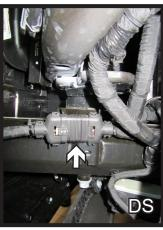
Remove fascia and set aside to be reinstalled later. Unplug the electrical on both sides of the vehicle as the fascia is removed.
