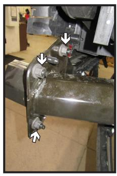
7. Using an 18MM socket or wrench, remove the three (3) nuts from the bumper. Do this on both sides of the vehicle. Remove bumper, it will not be reinstalled.
