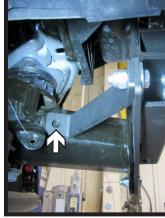
12. Using a 1/2" drill bit, drill the bottom inside hole on the front of the baseplate (left). Then using the support bracket as a template, drill 1/2" hole in frame (right). Do this on both sides of the vehicle.
