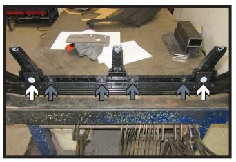
8. Using a 10MM socket, remove the two (2) bolts (white) from the plastic piece on the bottom of the bumper. Then using 1/4" drill bit, drill out the four (4) plastic rivets (gray). Remove plastic piece and set aside to be reinstalled with the baseplate.
