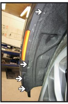
1. Using an 8MM socket, remove the four (4) bolts from the wheel well edge. Do this on both sides of the vehicle.
