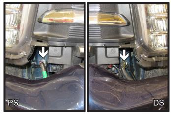
12. Disconnect the indicated wire loom on the driver side of the vehicle and the main wire loom on the passenger side of the vehicle. Remove bumper and set aside to be reinstalled later.
