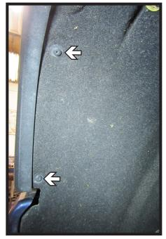
4. Using a T15 Torx, remove the two (2) bolts from along the edge of the wheel well. Do this on both sides of the vehicle.
