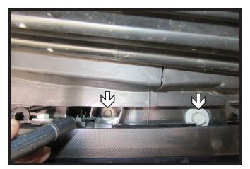
On the top side of the bumper, use an 18MM socket and socket extension to remove the two (2) bolts from behind the bumper. Do this on both sides of the vehicle.
