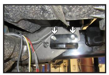
15. Slide the baseplate safety cable bracket onto the two (2) 1/2" bolts and place a nylon lock nut on each bolt to secure. Do this on both sides of the vehicle.
