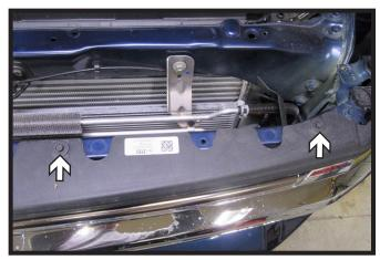
3. Using a 10MM socket, remove the two (2) bolts from the top of the fascia. Do this on both sides of the vehicle.
