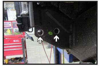
13. Using a 13/16" drill bit, drill out the two (2) tow hook holes. Do this on both sides of the vehicle.
