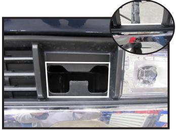
Trim the tow hook opening as indicated to allow room for the baseplate. Then trim the bottom inner side at an angle as needed (inset).
