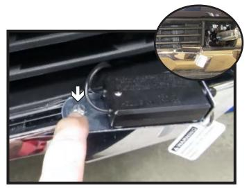
21. Optional: Using a 1/4" drill bit, drill one
