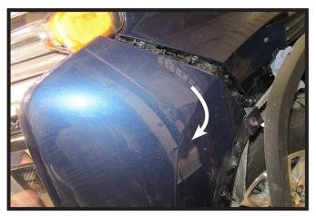
6. Grab fascia in the wheel well and pull outward firmly to remove corner of center fascia piece. Do this on both sides of the vehicle. Remove center fascia piece and set aside to be reinstalled later.
