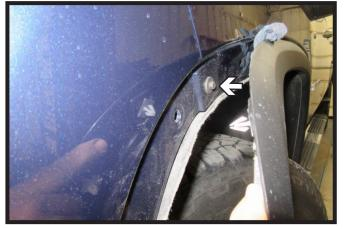
Unclip the front half of the wheel well trim. Prop trim away from vehicle using a rag or soft material to prevent scratching. Using a 7MM socket, remove the one (1) bolt from the fascia joint. Do this on both sides of the vehicle.
