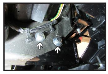
6. Insert two (2) 1/2" bolts with flat washers and spacers. Do this on both sides of the vehicle.
