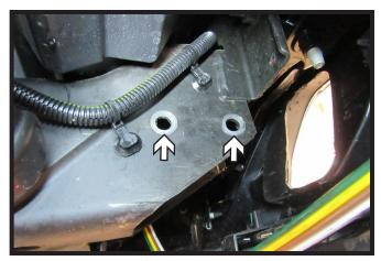
3. Using a 13/16" drill bit, drill out the two (2) holes on the inside of the frame only. Do this on both sides of the vehicle.
