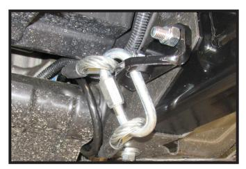
9. Attach the permanent baseplate safety cables to the provided convenience link on the baseplate. The photo above shows the recommended installation of the cables to frame of vehicle. Additional options may interfere with suggested mounting; in this case, secure the cables to a solid piece of the frame as described in the General Information sheet. Be sure the safety cables do not rub against any hoses or moving parts. Do this on BOTH sides of the vehicle.
