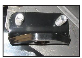
7. Slide the baseplate safety cable bracket onto the two (2) 1/2" bolts and place a nylon lock nut on each bolt to secure. Do this on both sides of the vehicle.
