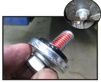
8. Start the one (1) 1/2" x 1-1/2" bolt with sleeve and hardware into the bottom hole. Do this on both sides of the vehicle.
