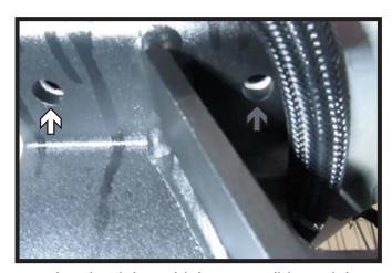
13. Slide the passenger side plate onto the vehicle ensuring that it is as high as possible and the front side is against the flange on the frame. Hold in place with vise grips. Using a 3/8" drill bit, drill the top three (3) holes and back bottom hole using the baseplate as a template (white). Mark the front bottom hole. Remove passenger side plate and using 3/8" drill bit, drill marked front bottom hole (gray). Reinstall passenger side plate using five (5) 3/8" bolts and hardware.
