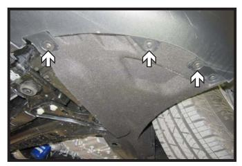
Using a T15 Torx, remove the six (6) bolts from the underside of the vehicle in front of the tire. There are three (3) on each side.
