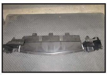
18. Using a utility knife, remove the side pieces as indicated from the plastic shroud. Reinstall shroud using the bottom three (3) existing bolts.
