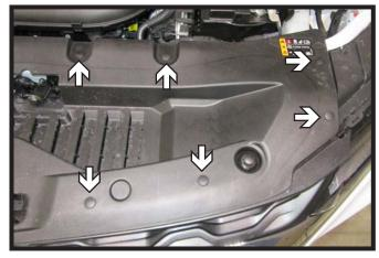
Remove the twelve (12) push pins from the fascia cover, there are six (6) on each side of the vehicle. Remove and set fascia cover aside to be reinstalled later.
