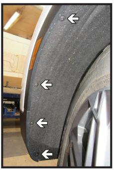
3. Using a T15 Torx, remove the four (4) bolts from the wheel well edge in front of the tire. Do this on both sides of the vehicle.
