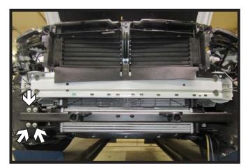
16. Install the remaining three (3) 3/8" bolts with hardware attaching the cross member to the passenger side plate.
