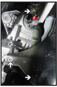
8. Pull back the wheel well liner. Using a 7MM socket, remove the three (3) bolts from behind the light. Do this on both sides of the vehicle.
