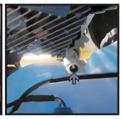
11. Using a 10MM socket, remove the three (3) bolts (white) and one (1) nut (gray) from the windshield washer fluid reservoir on the driver side of the vehicle. Disconnect and plug all lines. Remove reservoir and set aside to be reinstalled later.
