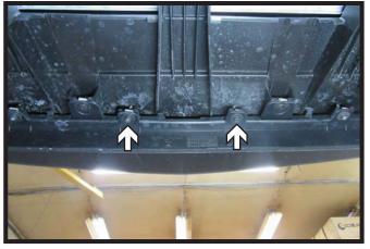
Using a 7MM socket, remove the two (2) bolts from the underside of the vehicle in the center.
