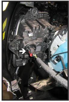
Pull the fascia away from the vehicle to unsnap. Unplug headlight on both sides of the vehicle, remove the fascia and set aside to be reinstalled later.
