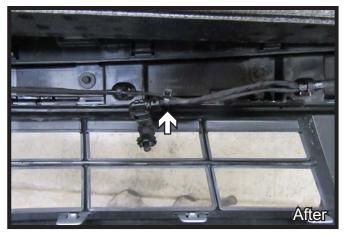
12. Remove the temperature sensor from the bracket on the back side of the fascia. Using a reciprocating saw, cut the bracket as shown. Relocate temperature sensor, connecting it to upper loom using two (2) provided zip ties.
