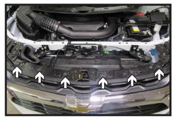
2. Using a T15 Torx, remove the six (6) bolts, three (3) on each side, from the top of the fascia.
