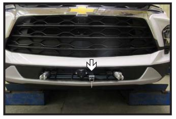
21. **Optional**: Install the breakaway to the electrical bracket with one (1) 1/4" bolt with hardware.
