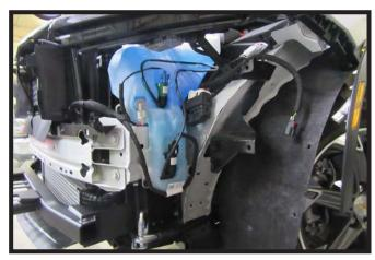
19. Reinstall the windshield washer fluid reservoir on the driver side of the vehicle. Reconnect all lines.
