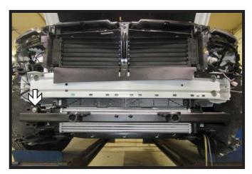
14. Hold the driver side plate and cross bar in place. Where the cross bar attaches to the passenger side plate, start one (1) 3/8" bolt and hardware. Use a vise grip to hold the driver side plate in place.
