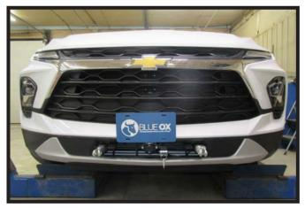
20. Hold the fascia as close to its original position, mark and trim the fascia around the convenience links and attachment tabs. Reinstall the fascia and fascia cover. Reconnect all electrical connections.
