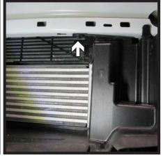
10. Using a 7MM socket, remove the five (5) bolts from the plastic shroud. There is one (1) on each side and three (3) under the vehicle. Remove shroud and set aside to be reinstalled later.
