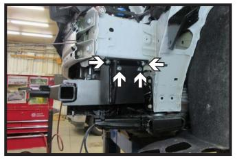
15. Using a 3/8" drill bit, drill the four (4) holes on the driver side of the vehicle using the end plate as a template. Then install four (4) 3/8" bolts with hardware.
