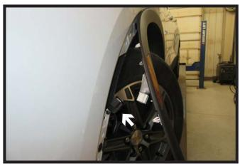
4. Unsnap the fender trim by pulling outward away from the fascia. Unplug the electrical. Place a rag or soft item between the trim and fascia to hold trim out of the way and prevent damage to the fascia. Do this on both sides of the vehicle.
