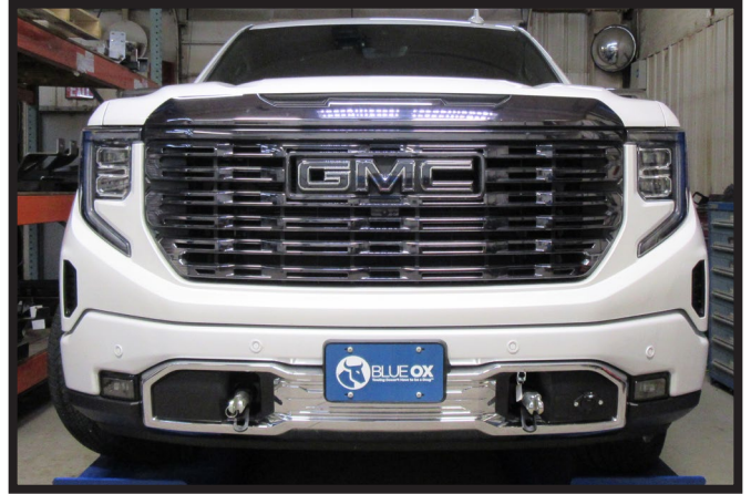
7b. Reinstall the bumper, grille, fascia, fascia cover. Reconnect all electrical and hoses.
