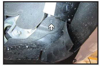
Using an 8MM socket, remove the one (1) bolt on the underside of the fascia in front of the tire. Do this on both sides of the vehicle.
