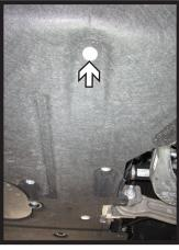
7. Using a 10MM socket, remove the two (2) bolts, one (1) on each side, from the belly pan.
