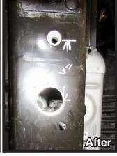
14. Measure 3" from the center of the top hole down. Using a 1-1/4" hole saw, drill hole centering hole with existing holes on the frame and the bottom of the 3" measurement. Do this on both sides of the vehicle.
