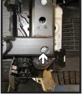
17. Install a 10MM x 1.5" bolt with flat washer and lock washer into bottom hole on each side of the vehicle.
