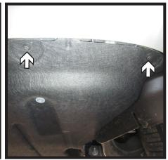
6. Using an 8MM socket, remove the five (5) bolts from the belly pan.
