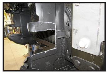
15. Using a reciprocating saw, trim the plastic shroud as indicated. Do this on both sides of the vehicle.
