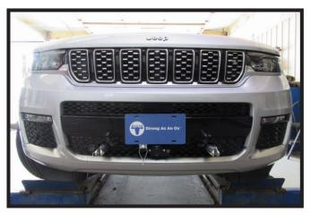
23. Hold the fascia as close to its original position, mark and trim the fascia around the convenience links and attachment tabs. Reinstall the fascia, fascia cover, and belly pan. Reconnect all electrical connections and windshield washer fluid line.
