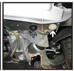
9. Let belly ban hang. Using a 10MM socket, remove the four (4) bolts (white) from the underside of the fascia. Then remove the two (2) push pins (gray).
