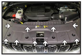
Remove the ten (10) push pins from the top of the fascia cover. Remove fascia cover and set aside to be reinstalled later.
