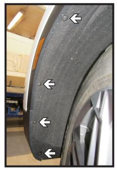
3. Using a T15 Torx, remove the four (4) bolts from the wheel well edge in front of the tire. Do this on both sides of the vehicle.
