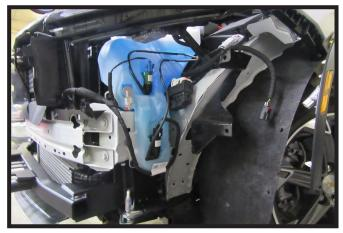
Reinstall the windshield washer fluid reservoir on the driver side of the vehicle. Reconnect all lines.
