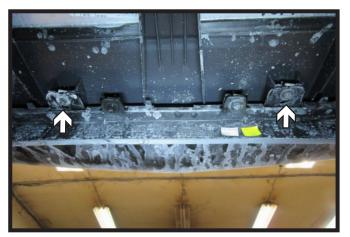
7. Using a 7MM socket, remove the two (2) bolts from the underside of the vehicle in the center.
