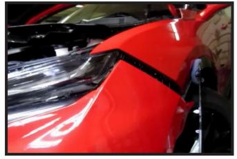
Pull the fascia away from the vehicle to unsnap. Unplug all electrical connections, remove the fascia and set aside to be reinstalled later.
