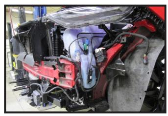
22. Reinstall the windshield washer fluid reservoir on the driver side of the vehicle. Reconnect all lines.
