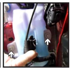
10. Using a 10MM socket, remove the four (4) bolts from the windshield washer fluid reservoir on the driver side of the vehicle. Disconnect all lines. Remove reservoir and set aside to be reinstalled later.
