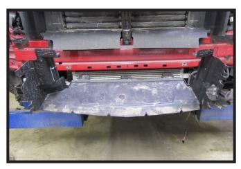
21. Hold plastic shroud in place, mark, and trim as needed around baseplate before reinstalling.
