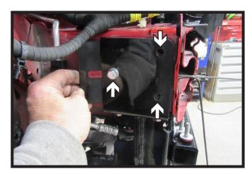
18. Start the three (3) remaining 3/8" bolts with hardware on the passenger side of the vehicle. Insert shim as shown and tighten all hardware. Reinstall the two (2) bumper bolts.
