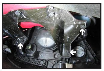
8. Pull back the wheel well liner. Using a 7MM socket, remove the three (3) bolts from behind the light. Do this on both sides of the vehicle.
