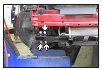
19. Install the remaining three (3) 3/8" bolts with hardware attaching the cross member to the passenger side plate.
