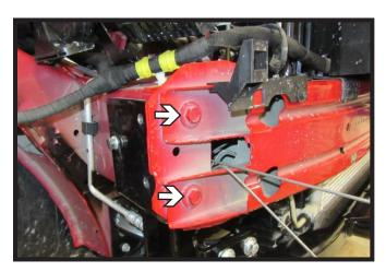
17. Using a 15MM socket remove the two(2) bolts from the bumper to allow room to install the bolts on the passenger side plate. Set aside to be reinstalled later.
