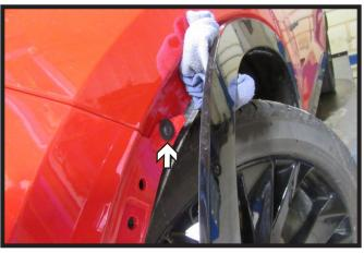
5. Using a T15 Torx, remove the one (1) bolt from the fascia joint under the fender trim. Do this on both sides of the vehicle.
