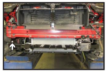
14. Hold the driver side plate and cross bar in place. Where the cross bar attaches to the passenger side plate, start one (1) 3/8" bolt and hardware. Use a vise grip to hold the driver side plate in place.
