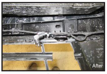
23. Remove the temperature sensor from the bracket on the back side of the fascia. Using a reciprocating saw, cut the bracket as shown. Relocate temperature sensor, connecting it to upper loom using two (2) provided zip ties.
