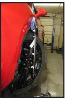
4. Unsnap the fender trim by pulling outward away from the fascia. Place a rag or soft item between the trim and fascia to hold trim out of the way and prevent damage to the fascia. Do this on both sides of the vehicle.
