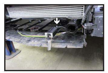
24. **Optional**: Install the breakaway to the bracket on the baseplate with one (1) 1/4" bolt with hardware.
