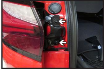
Using a 7MM socket, remove the two (2) bolts attaching the tail light to the frame.
