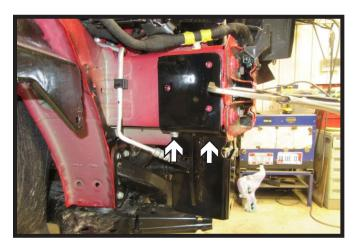
13. Slide the passenger side plate onto the vehicle ensuring that it is as high as possible and as far forward as possible. Using a 3/8" drill bit, drill the two (2) bottom holes and start the two (2) 3/8" bolts with hardware.
