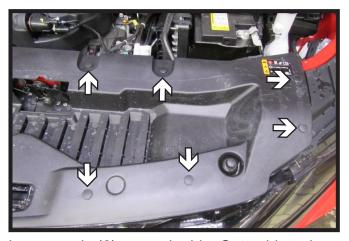
1. Remove the twelve (12) push pins from the fascia cover, six (6) on each side. Set aside to be reinstalled later.
