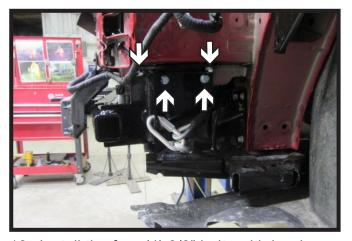
16. Install the four (4) 3/8" bolts with hardware on the driver side of the vehicle.
