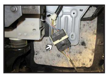
7. As the fascia is removed, unplug the electrical connection on the driver side of the vehicle. Remove fascia and set aside to be reinstalled later.
