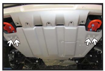
3. **Tremor Models**: Using a 13MM socket, remove the four (4) bolts from the belly pan, there are two (2) bolt on each side.
