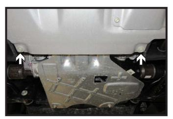
4. **Tremor Models**: Using a 15MM socket, loosen the back two (2) bolts of the belly pan. Slide belly pan off the vehicle and set aside to be reinstalled later.
