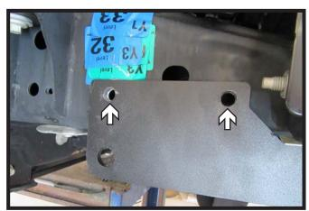
4. Using a 1/2" drill bit, drill two (2) holes in the side of the frame using the baseplate as a template. Do this on both sides of the vehicle.
