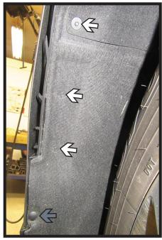
1. Using a 5.5MM socket remove the three (3) bolts (white) and one (1) push pin (gray) from the wheel well edge. Do this on both sides of the vehicle.
