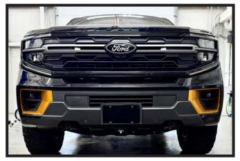
8d. **2025 Tremor Models:** Reinstall fascia, belly pan and belly pan brackets. Reconnect electrical connection on the driver side of the vehicle.
