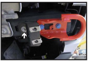
7. Using a 13MM socket, remove the one (1) bolt from the belly pan bracket. Remove bracket and set aside to be reinstalled later. Do this on both sides of the vehicle.
