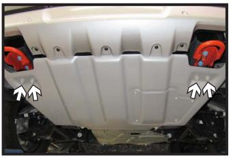
5. Using a 13MM socket, remove the four (4) bolts from the belly pan, there are two (2) bolt on each side.
