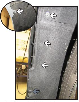
1. Using a 5.5MM socket remove the four (4) bolts (white) and one (1) push pin (gray) from the wheel well. Do this on both sides of the vehicle.
