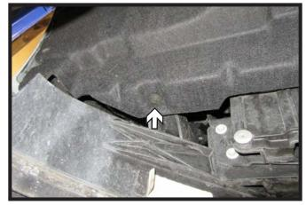
Using a 5.5MM socket, remove the one
