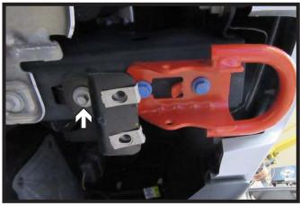
5. Using a 13MM socket, remove the one (1) bolt from the belly pan bracket. Remove bracket and set aside to be reinstalled later. Do this on both sides of the vehicle.
