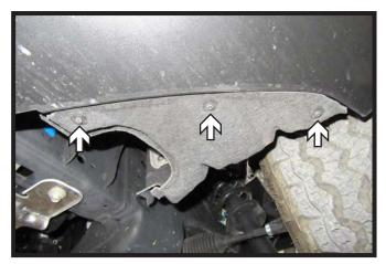
Using a 5.5MM socket, remove the three
