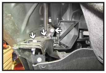
2. Pull back the wheel well liner back. Using a 10MM socket remove the three (3) bolts. Do this on both sides of the vehicle.
