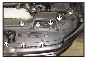
1. Remove the thirteen (13) push pins from the top of the fascia. Remove fascia cover and set aside to be reinstalled later.
