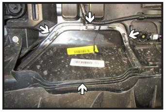
7b. **2025 Models Only:** Remove the four (4) clips attaching the tow hook cover to the fascia. Push cover inward to remove. Set cover aside, it will not be reinstalled. Do this on both sides of the vehicle.
