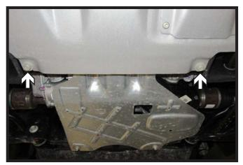
Using a 15MM socket, loosen the back two (2) bolts of the belly pan. Slide belly pan off the vehicle and set aside to be reinstalled later.
