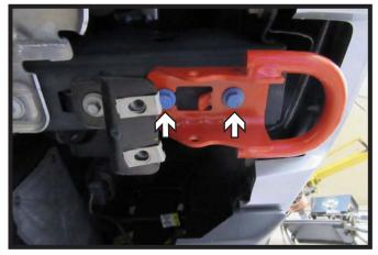
Vehicles with Tow Hooks: Using a 15MM socket, remove the two (2) bolts from the tow hook. Remove tow hook, it will not be reinstalled. Do this on both sides of the vehicle.
