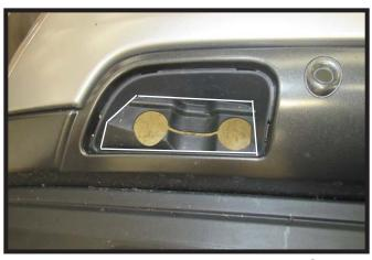
7a. **2018-24 Non-Timberline Models Only:**Remove the area shown to allow room for the tab and convenience link. Do this on both sides of the vehicle.
