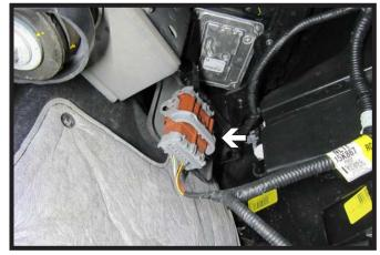
2018-2024 Models: Disconnect electrical connection on the driver side of the vehicle.
