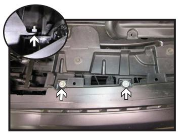
Using a 10MM socket, remove the two (2) bolts from the top of the fascia and one (1) nut (inset) from behind the head light. Do this on both sides of the vehicle.
