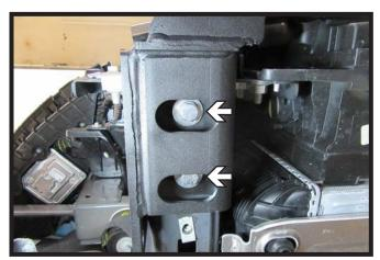
3. Hold baseplate in position and start two (2) 1/2" x 1-3/4" bolts with flat washers, lock washers, and whiz nuts. Push baseplate flush against the frame and hand tighten bolts. Do this on both sides of the vehicle.
