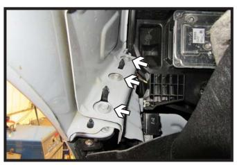
Pull back the wheel well liner. Using a 10MM socket remove the three (3) bolts from the fascia joint. Do this on both sides of the vehicle.
