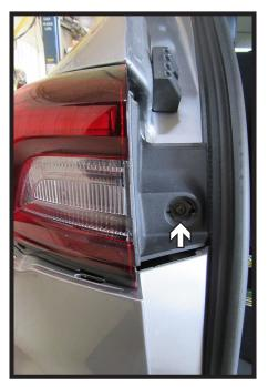
5. Using a T25 Torx, remove the two (2) bolts from the tail light housing. Remove housing and install tail light wiring kit per manufactures instructions. Reinstall tail light housing, rear panel and push pins. Do this on both sides of the vehicle.
