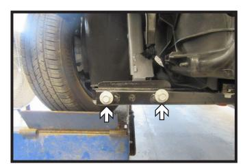
9. Using a 13MM socket, remove the two (2) bolts from the cross bar. Do this on both sides of the vehicle.
