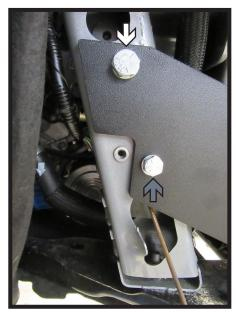
18. Insert nut plate through hole in the frame (left). Insert a 1/2" bolt with lock washer into the top hole (white) and a 3/8" bolt with lock washer into the bottom hole (gray). Do this on both sides of the vehicle.
