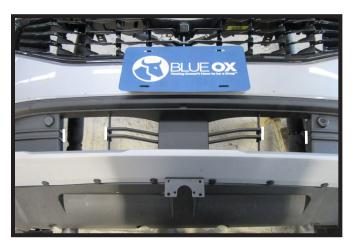
24. Remove the two (2) horizontal slats between the white marks as shown to allow room for the removable tabs and convenience links.
