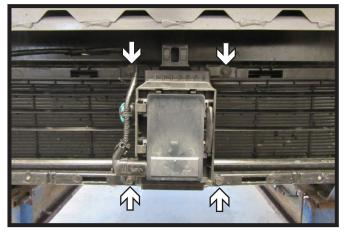
Using an 8MM socket, remove the four (4) bolts attaching the Adaptive Cruise Control (ACC) to the vehicle. Let hang out of the way for baseplate installation but DO NOT unplug sensor.
