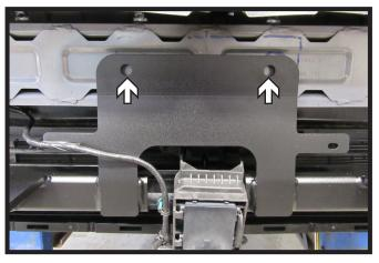
13. Using a 1/2" drill bit, drill out the two (2) holes as shown using the baseplate as a template.
