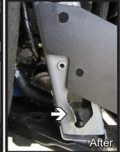
17. Using a pair of large vise grips bend back the frame piece as shown to create an access hole for the nut plate. Do this on both sides of the vehicle.
