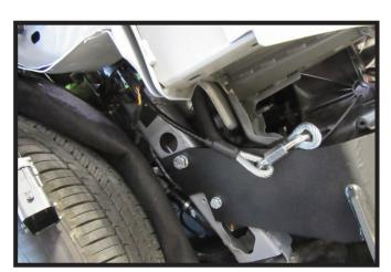
22. Attach the permanent baseplate safety cables to the provided convenience link on the baseplate. The photo above shows the recommended installation of the cables to frame of vehicle. Additional options may interfere with suggested mounting; in this case, secure the cables to a solid piece of the frame as described in the General Information sheet. Be sure the safety cables do not rub against any hoses or moving parts. Do this on **BOTH** sides of the vehicle.
