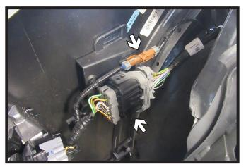
Disconnect the two (2) electrical connections on the passenger side of the vehicle. Remove fascia and set aside to be reinstalled later.
