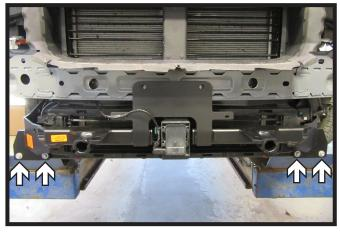
12. Slide the baseplate onto the vehicle and reinstall the four (4) existing 8MM bolts and washers, two (2) on each side. Use level to ensure baseplate is level before tightening bolts.
