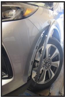
3. Pull back the wheel well trim past the fascia joint and hold in place with a soft cloth. Do this on both sides of the vehicle.
