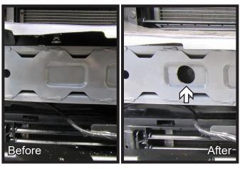
14. Using a 1-1/4" hole saw, drill out the hole as shown to create access hole. Do this on both sides of the vehicle.
