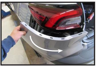
Remove the rear panel below the tail light housing. Do this on both sides of the vehicle.
