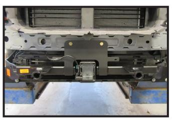
19. Reinstall the four (4) bolts attaching the ACC to the frame.
