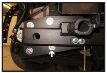
15. Install one (1) 1/2" x 1-1/2" bolt with flat washer and nylon lock nuts into the bottom inside hole on the front of the baseplate. Do this on both sides of the vehicle.
