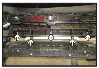
Using a 13MM socket, remove the five (5) nuts on the backside of the fascia. Remove foam piece and set aside. It will not be reinstalled.
