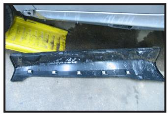
10. Using a flat screwdriver, pry the black covering piece off of each of the five (5) tabs below the door panel. Do this on both sides of the vehicle.
