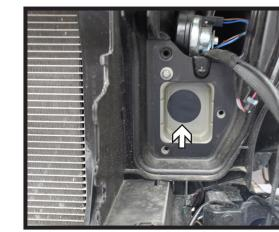
20. Peel off the tape covering the frame hole to allow nut plate access for baseplate installation. Do this on both sides of the vehicle.
