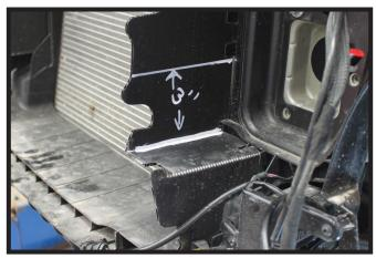
21. Using the utility knife, cut a piece 3" wide from the middle of the corrugated plastic. This will allow the baseplate to slide on.
