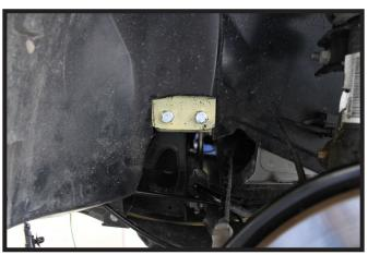
33. Trim the lower portion of the inner wheel well as shown to allow the wheel well to be reinstalled to its original position.
