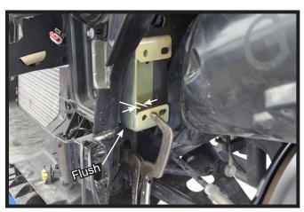
23. Align the support bracket, 1/4" from the backside of the bumper lip and flush with the bottom of the frame and clamp into position. Do this on both sides of the vehicle.
