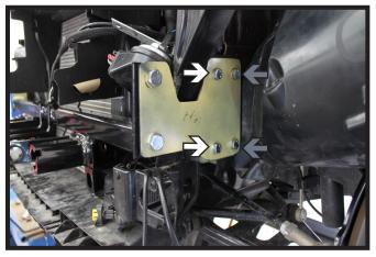
26. Loosely attach the support bracket to the end plate. Use 3/8"-16 x 1-1/4" bolts with 3/8" lock washers (gray) and 3/8"-16 nut plates. On the front holes, use 3/8"-16 x 1-1/4" bolts with 3/8" lock washers and 3/8" whiz nuts. Do this to both sides of the vehicle.
