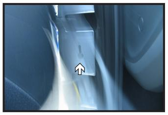
6. Lower on the inside of the door, remove the push pin. Do this on both sides of the vehicle.
