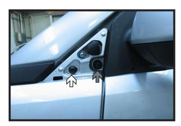
Using the 25 Torx, remove the front bolt next to the antenna (white). Then remove the rear bolt using a 30 Torx (gray).
