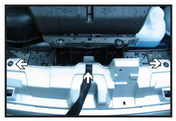
Using a T25 Torx, remove the three (3) screws from the top edge of the fascia.
