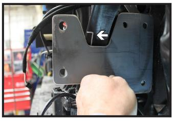
25. Line up the bolt holes of the support bracket and side plate by hand and mark a notch. This notch needs to provide enough clearance to allow the side plate to be installed.
