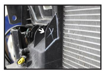
28. On the passenger side, trim off the tab using the outer edge as a guide.
