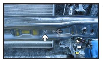
19. Using the 3/8" 12 point socket, remove the four (4) bolts holding the bumper. Do this on both sides of the vehicle. Set the bumper aside.
