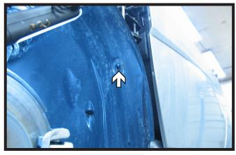
17. Remove the push pin on the right side. Do this on both sides of the vehicle. Pull the wheel well covers out of the way.
