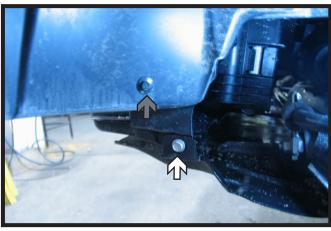
14. Using a 10MM socket, remove the bolt on the wheel well at the front. Remove the push pin above, (gray). Do this on both sides of the vehicle.
