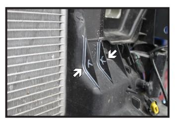
27. On the driver side of the vehicle, use a utility knife to remove the two (2) gussets.
