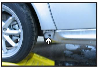
11. Using the 25 Torx, remove the bolt holding the fascia just behind the front tire. Do this on both sides of the vehicle.
