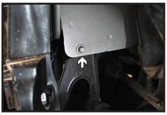
22. **2012-15 models only:** Using a 5/16" 12 point socket remove the bolt on both sides of the vehicle. Replace with the 6MM-1.0 x 16MM bolts that are included in the baseplate bolt bag. Be sure the sides of the bolt head are vertical so the bracket will slide on easily.
