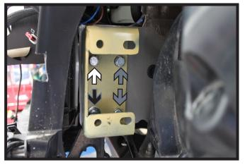
24. Using the support bracket holes as a template, drill four (4) holes thru the frame with a 13/32" drill bit. Use two (2) 3/8"-16 x 1-1/4" bolts with 3/8" lock washers and 3/8"-16 nut plates in the rear holes (gray). Use a 3/8"-16 x 1-1/4" bolt with 3/8" lock washer and 3/8"-16 whiz nut in top front hole (white). Use a 3/8"-16 x 1-1/4" bolt with 3/8" lock washer, 3/8" flat washer and 3/8"-16 whiz nut in bottom front hole (black). Do this to both sides of the vehicle.
