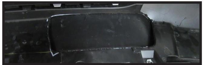
8. Using a reciprocating saw, trim the marked areas on the fascia, ensuring to not cut completely through the fascia.
