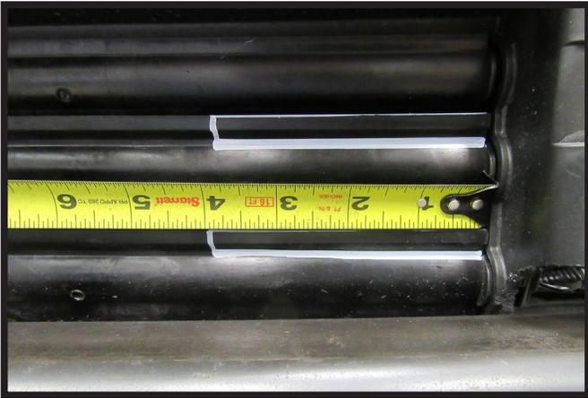
9. Using a reciprocating saw, trim the bottom two shutters, 4" across and roughly 1/2" deep. Do this for both sides of the vehicle.
