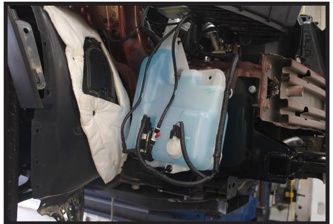
17. Install nine (9) 1/4" washers onto the two (2) studs for the washers reservoir (top). Reinstall the washer reservoir onto the studs and reinstall the factory nuts. The factory screw will not be reinstalled.
