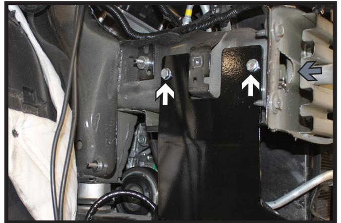
15. Using a 3/8" drill bit, drill the upper two (2) holes on the side of the baseplate thru the frame. Install the 3/8" bolts (white) as indicated and insert wire nuts through the hole in the frame (gray), fully tighten. Do this on both sides of the vehicle.
