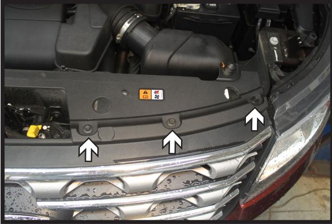
1. Using a 10MM socket, remove the seven (7) screws from the top edge of the fascia. There are three (3) on the driver side and four (4) on the passenger side.
