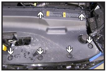
1. Remove the twelve (12) push pins from the fascia cover. There are six (6) on each side. Set cover aside to be reinstalled later.
