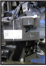
19. Using a utility knife, trim the bumper cover on both sides of the vehicle as indicated to allow clearance for the baseplate.
