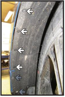
Using a 5.5MM socket, remove the four
