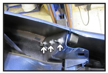
Using an 8MM socket, remove the three
