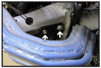
13. Install the baseplate onto the frame with the provided 3/8" hardware, making sure to not yet fully tighten the hardware. Do this on both sides of the vehicle.
