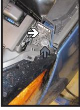
3. Using a 10MM socket, remove the two (2) bolts (white) from the headlight. Then remove the one (1) push pin (gray). Disconnect all electrical connections and set the headlight aside to be reinstalled later. Do this on both sides of the vehicle.
