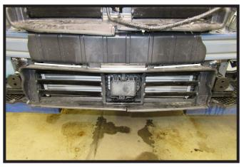
8. Using a 7MM wrench on backside (inset), remove the indicated bolt from the bottom of the shutter housing (left). Then using a utility knife cut along the top and around the edge of the housing as indicated (right). Unsnap the bottom of the shutter housing, remove, and set aside. It will not be reinstalled later.
