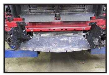
21. Hold plastic shroud in place, mark, and trim as needed around baseplate before reinstalling.
