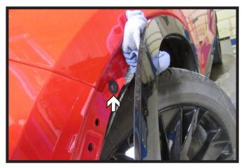
Using a T15 Torx, remove the one (1) bolt from the fascia joint under the fender trim. Do this on both sides of the vehicle.
