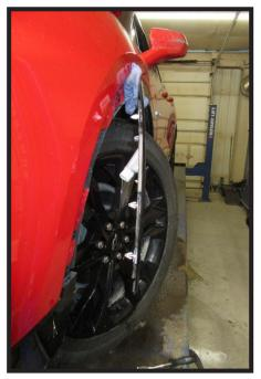
4. Unsnap the fender trim by pulling outward away from the fascia. Place a rag or soft item between the trim and fascia to hold trim out of the way and prevent damage to the fascia. Do this on both sides of the vehicle.
