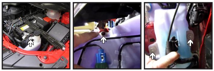
10. Using a 10MM socket, remove the four (4) bolts from the windshield washer fluid reservoir on the driver side of the vehicle. Disconnect all lines. Remove reservoir and set aside to be reinstalled later.
