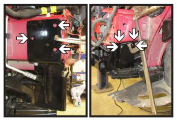
Using a 3/8" drill bit, drill the remaining seven (7) holes, four (4) on the driver side and three (3) on the passenger side. Use the end plates as templates.
