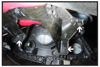
8. Pull back the wheel well liner. Using a 7MM socket, remove the three (3) bolts from behind the light. Do this on both sides of the vehicle.
