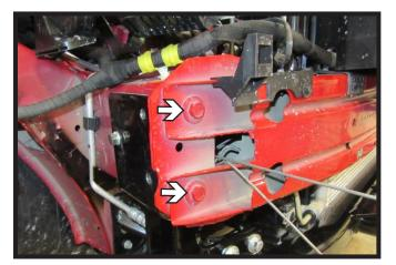
17. Using a 15MM socket remove the two(2) bolts from the bumper to allow room to install the bolts on the passenger side plate. Set aside to be reinstalled later.
