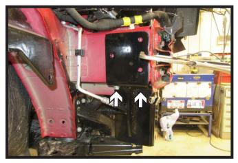
Slide the passenger side plate onto the vehicle ensuring that it is as high as possible and as far forward as possible. Using a 3/8" drill bit, drill the two (2) bottom holes and start the two (2) 3/8" bolts with hardware.
