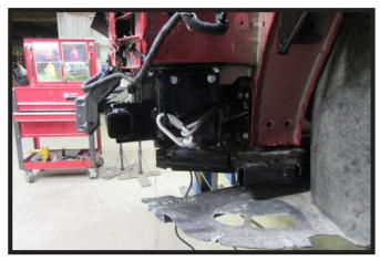
20. Attach the permanent baseplate safety cables to the provided convenience link on the baseplate. The photo above shows the recommended installation of the cables to frame of vehicle. Additional options may interfere with suggested mounting; in this case, secure the cables to a solid piece of the frame as described in the General Information sheet. Be sure the safety cables do not rub against any hoses or moving parts. Do this on **BOTH** sides of the vehicle.
