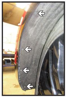
3. Using a T15 Torx, remove the four (4) bolts from inside of the wheel well in front of the tire. Do this on both sides of the vehicle.
