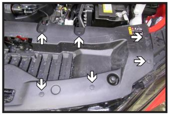
1. Remove the twelve (12) push pins from the fascia cover, six (6) on each side. Set aside to be reinstalled later.
