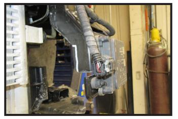
11. On the driver side of the vehicle use a reciprocating saw to trim the back of the Adaptive Cruise Control (ACC) bracket approximately 1/4 inch or more to allow clearance for the baseplate.
