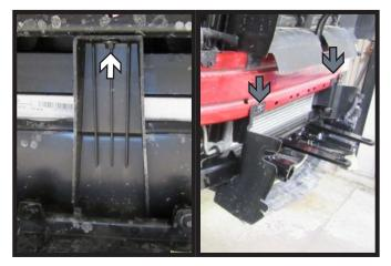
12. Using a 10MM socket, remove the three (3) bolts (white) on the underside of the vehicle holding the plastic shroud. Then using a 7MM socket, remove the two (2) bolts (gray) from above the shroud. Remove shroud and set aside to be reinstalled later.
