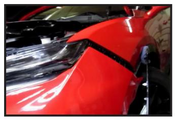
9. Pull the fascia away from the vehicle to unsnap. Unplug all electrical connections, remove the fascia and set aside to be reinstalled later.
