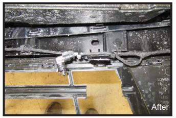
23. Remove the temperature sensor from the bracket on the back side of the fascia. Using a reciprocating saw, cut the bracket as shown. Relocate temperature sensor, connecting it to upper loom using two (2) provided zip ties.
