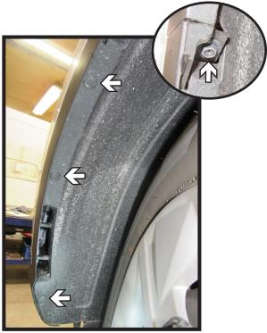
2. Remove the three (3) push pins along the edge of the wheel well. Then using an 8MM socket, remove the one (1) bolt from the fascia joint (inset). Do this on both sides of the vehicle.
