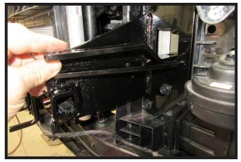
12. Slide frame support brace into place.
