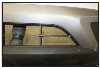
15. Remove the two (2) horizontal slats as shown on the driver side of the fascia to allow room for the removable tab, convenience link and electrical.
