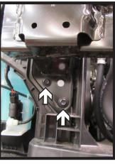
5. Using a 12MM socket, remove the four (4) bolts (white) from the bumper. Using a 10MM socket, remove the one (1) nut (gray) on the top of the bumper. Do this on both sides of the vehicle. Remove bumper, it will not be reinstalled later.
