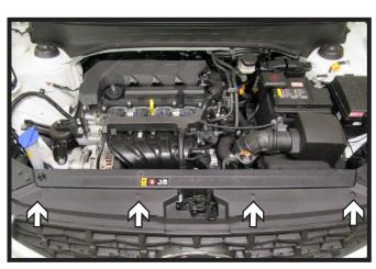
1. Remove the four (4) push pins along the top of the fascia.
