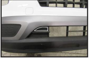
16. Remove the outer horizontal slat as shown on the passenger side of the fascia to allow room for the removable tab and convenience link.
