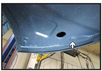
On the underside of the vehicle remove the indicated push pin. Do this on both sides of the vehicle.
