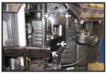
9. Lift baseplate to center rest of the holes. Reinstall the four (4) existing 10MM bolts on each side of the vehicle.
