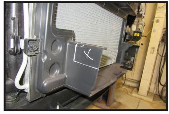
Trim the plastic piece on the passenger side of the vehicle as shown.
