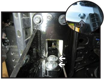
13. Install 3/8" bolts with flat washers and nylon lock nuts into the front two (2) holes (white). In the back hole install one (1) 1/2" bolt with lock washer, large flat washer, small flat washer from the bottom of the frame and a whiz nut through the frame opening (inset).
