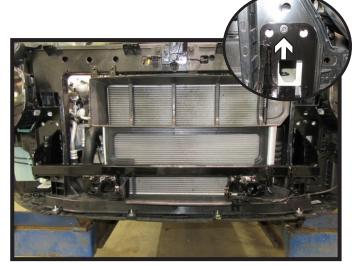
8. Slide the baseplate into place. Install the existing 5MM nut on both sides vehicle to hold the baseplate in place (inset).
