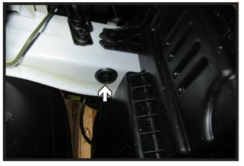
10. Remove the plastic plug from the bottom of the frame. Do this on both sides of the vehicle.
