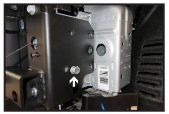
19. Start a 1/2" x 1-1/2" bolt with lock washer and whiz nut in the bottom front hole. Leave loose at this time. Do this on both sides of the vehicle
