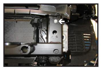
16. Hold baseplate into place on the vehicle frame and start the existing bolt in the top hole. Do this on both sides of the vehicle. **Note:** Ensure all holes line up before tightening bolts.
