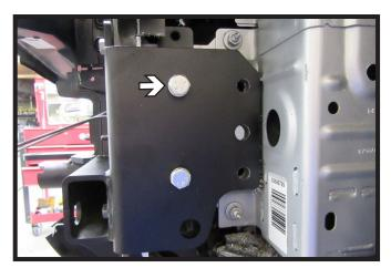
20. Insert spacer plate at top of baseplate between the frame and baseplate with the slotted end facing downward. Once spacer plate is in position insert 1/2" x 1-1/2" bolt with lock washer and whiz nut into top front hole. Do this on both sides of the vehicle.
