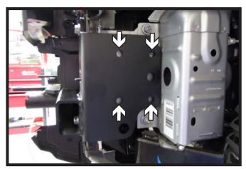
18. Using 1/2" drill bit. Drill the four (4) holes on the side of the frame using the baseplate as a template. Do this on both sides of the vehicle
