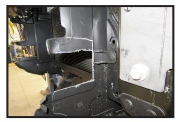
15. Using a reciprocating saw, trim the plastic shroud as indicated. Do this on both sides of the vehicle.
