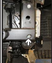
17. Install existing bolt into bottom hole on each side of the vehicle.
