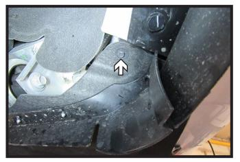
8. Using an 8MM socket, remove the one (1) bolt on the underside of the fascia in front of the tire. Do this on both sides of the vehicle.
