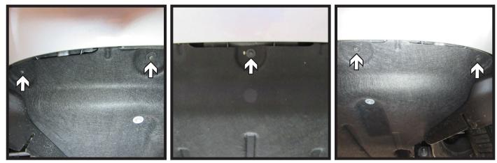
6. Using an 8MM socket, remove the five (5) bolts from the belly pan.
