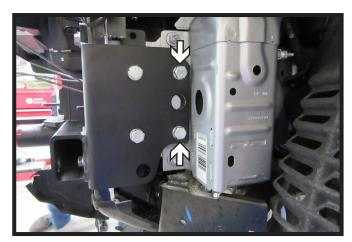
21. Install two (2) 1/2" x 1-1/2" bolts with lock washers and whiz nuts back holes. Do this on both sides of the vehicle. Tighten all bolts at this time.
