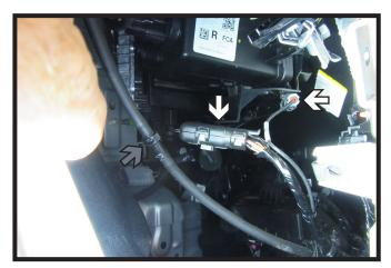
Unplug two (2) electrical connections (white) on the passenger side of the vehicle. Then disconnect windshield washer fluid line (gray).
