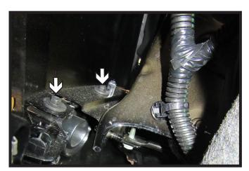
6. Pull back the wheel well liner. Using a 10MM socket, remove the two (2) bolts as indicated. Do this on both sides of the vehicle.
