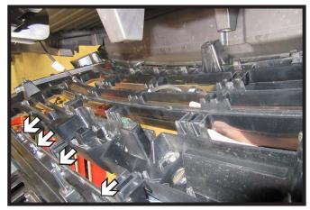
9. Reach from the top inside of the vehicle to release the four (4) clips connecting the center section of the fascia to the frame. Remove fascia and set aside to be reinstalled later.
