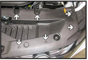
1. Remove the twelve (12) push pins from the fascia cover, there are six (6) on each side of the vehicle. Remove and set fascia cover aside to be reinstalled later.
