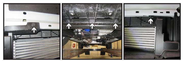
10. Using a 7MM socket, remove the five (5) bolts from the plastic shroud. There is one (1) on each side and three (3) under the vehicle. Remove shroud and set aside to be reinstalled later.
