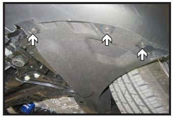
6. Using a T15 Torx, remove the six (6) bolts from the underside of the vehicle in front of the tire. There are three (3) on each side.
