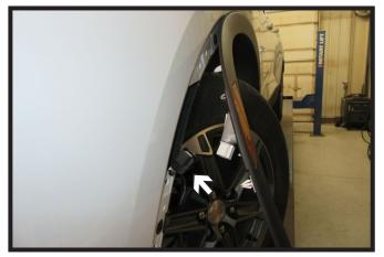
4. Unsnap the fender trim by pulling outward away from the fascia. Unplug the electrical. Place a rag or soft item between the trim and fascia to hold trim out of the way and prevent damage to the fascia. Do this on both sides of the vehicle.
