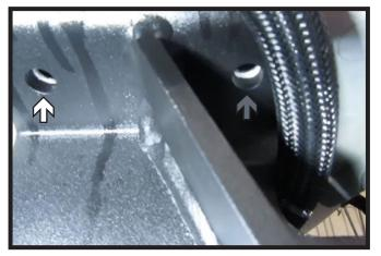
13. Slide the passenger side plate onto the vehicle ensuring that it is as high as possible and the front side is against the flange on the frame. Hold in place with vise grips. Using a 3/8" drill bit, drill the top three (3) holes and back bottom hole using the baseplate as a template (white). Mark the front bottom hole. Remove passenger side plate and using 3/8" drill bit, drill marked front bottom hole (gray). Reinstall passenger side plate using five (5) 3/8" bolts and hardware.
