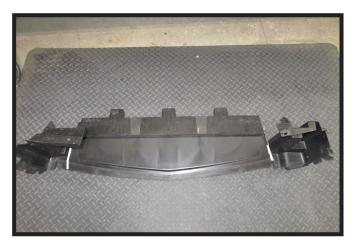
Using a utility knife, remove the side pieces as indicated from the plastic shroud. Reinstall shroud using the bottom three (3) existing bolts.
