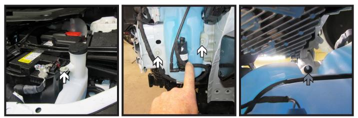
11. Using a 10MM socket, remove the three (3) bolts (white) and one (1) nut (gray) from the windshield washer fluid reservoir on the driver side of the vehicle. Disconnect and plug all lines. Remove reservoir and set aside to be reinstalled later.
