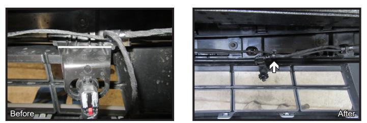
12. Remove the temperature sensor from the bracket on the back side of the fascia. Using a reciprocating saw, cut the bracket as shown. Relocate temperature sensor, connecting it to upper loom using two (2) provided zip ties.
