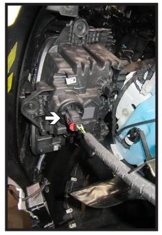
9. Pull the fascia away from the vehicle to unsnap. Unplug headlight on both sides of the vehicle, remove the fascia and set aside to be reinstalled later.
