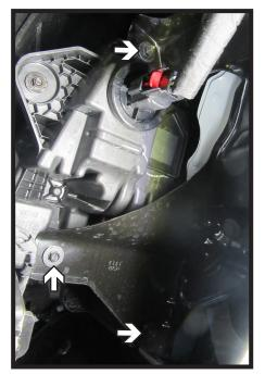
Pull back the wheel well liner. Using a 7MM socket, remove the three (3) bolts from behind the light. Do this on both sides of the vehicle.
