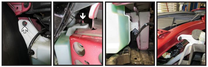
12. Using a 10MM socket, remove the two (2) nuts (white), one (1) bolt (gray), and one (1) push pin (black) from the windshield washer fluid reservoir on the passenger side of the vehicle. Disconnect and plug all lines. Remove reservoir and set aside to be reinstalled later.
