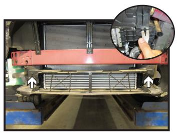
8. Remove the two (2) push pins, one (1) on each side from the plastic shroud. Then release clip from the bottom of shroud on each side (inset). Remove shroud and set aside, it will not be reinstalled.
