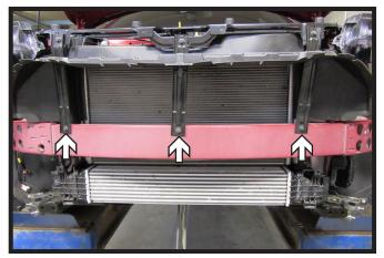
Using a 10MM socket, remove the three (3) bolts from the bumper support brackets. Remove bumper and set aside to be reinstalled later.
