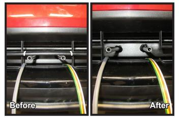
27. Using a reciprocating saw, trim the horizontal rib on the fascia as shown to allow room for the electrical plug.
