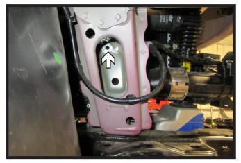
Using a 1/4" drill bit, create starter hole in frame on the passenger side of the vehicle. Then using a 1/2" drill bit, drill out top hole in frame.
