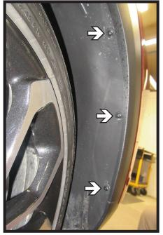
2. Using a T15 Torx, remove the three (3) bolts from the wheel well edge. Do this on both sides of the vehicle.
