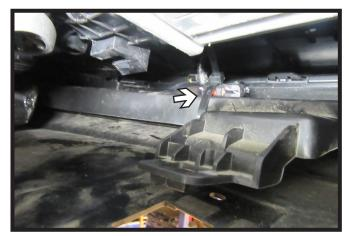
Start reinstalling the fascia. Before reinstalling bottom bolts, relocate and secure temperature sensor using provided 9" zip tie.
