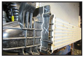
10. Using a reciprocating saw, trim the plastic as shown for baseplate clearance. Do this on both sides of the vehicle.
