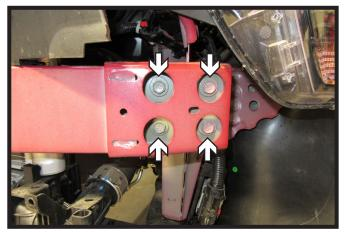
Using a 15MM socket, remove the four
