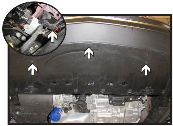
7. Using a T15 Torx, remove the three (3) bolts from the bottom of the fascia. Then disconnect the electrical on the driver side of the vehicle (inset). Remove fascia and set aside to be reinstalled later.
