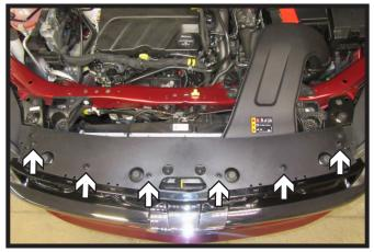
1. Using a T15 Torx, remove the six (6) bolts from the top edge of the fascia. There are three (3) on each side.
