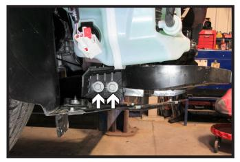
Using a 13MM socket, remove the two (2) bolts from plastic piece below the windshield washer reservoir. Do this on both sides of the vehicle. Remove piece and set aside to be reinstalled later.
