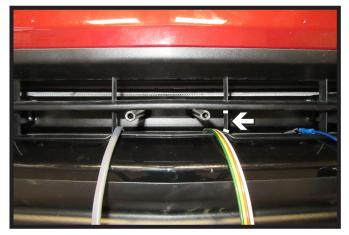
26. **Optional Breakaway**: Using a reciprocating saw, trim bottom vertical rib on the fascia as indicated to allow clearance for the breakaway bracket.
