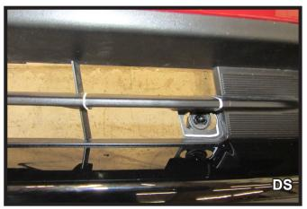
25. Unclip temperature sensor from the bracket on the back of the fascia. Then using a reciprocating saw trim each side of the fascia as shown to allow room for the baseplate and convenience link.
