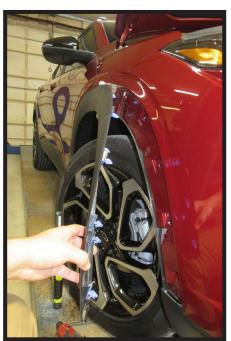
3. Pull back the wheel well trim, releasing the nine (9) push pins, past the fascia joint. Prop trim way from the vehicle using a soft cloth. Do this on both sides of the vehicle.
