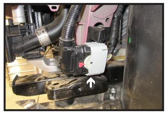
20. Unclip electrical loom from frame on driver side of the vehicle to allow for installation of support plate.
