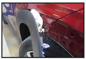
4. Using a 7MM socket, remove the one (1) bolt from the fascia joint. Do this on both sides of the vehicle.
