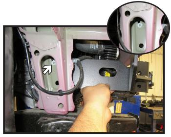
18. Hold the support plate in place as shown on passenger side of the vehicle so the front holes and back bottom hole line up with the existing holes on the vehicle. Mark frame using the baseplate as a template for top back hole.
