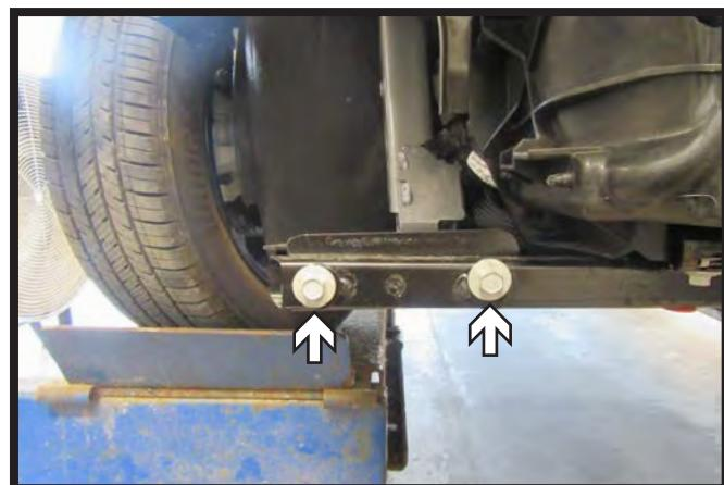
9. Using a 13MM socket, remove the two (2) bolts from the cross bar. Do this on both sides of the vehicle.
