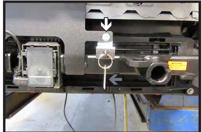
20. **Optional Breakaway:** Put a 90° bend in the breakaway bracket, 1-1/2" from the back and attach to the back of the electrical mounting bracket with provided 1/4" bolt, washers, and nut as shown. Remove white tag (gray) from breakaway switch so it does not interfere with any of the vehicle sensors.
