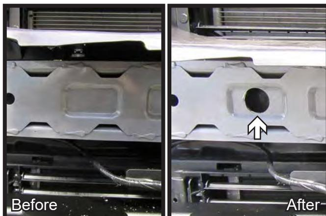
14. Using a 1-1/4" hole saw, drill out the hole as shown to create access hole. Do this on both sides of the vehicle.
