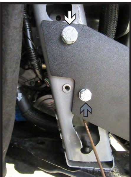
18. Insert nut plate through hole in the frame. Insert a 1/2" bolt with lock washer into the top hole (white) and a 3/8" bolt with lock washer into the bottom hole (gray). Do this on both sides of the vehicle.
