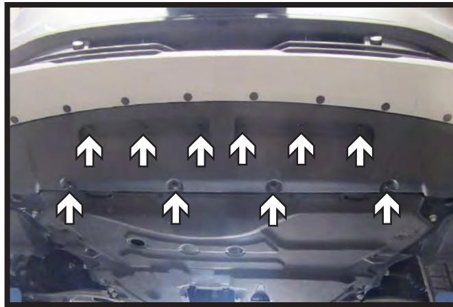
5. Using a T30 Torx, remove the ten (10) bolts from the bottom of the fascia.
