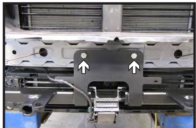
15. Install two (2) 1-1/2" bolts with washers and wire nuts. Torque bolts to 50 ft/lbs.
