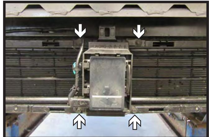
8. Using an 8MM socket, remove the four (4) bolts attaching the Adaptive Cruise Control (ACC) to the vehicle. Let hang out of the way for baseplate installation but DO NOT unplug sensor.
