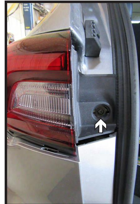
5. Using a T25 Torx, remove the two (2) bolts from the tail light housing. Remove housing and install tail light wiring kit per manufactures instructions. Reinstall tail light housing, rear panel and push pins. Do this on both sides of the vehicle.
