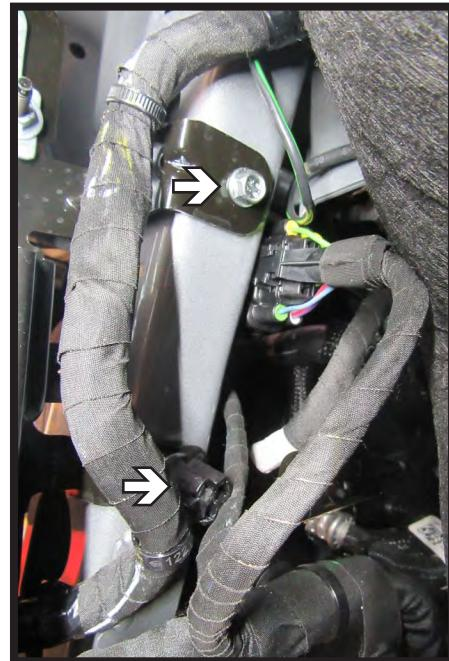
10. Using a 10MM socket, remove the one (1) bolt from the top of the black box in front of the wheel on the driver side of the vehicle (left). Then remove the wire loom from the backside bottom bolt. Using a 10MM deep socket, remove the two (2) bolts from the backside (right). Let box hang out of the way for baseplate installation.
