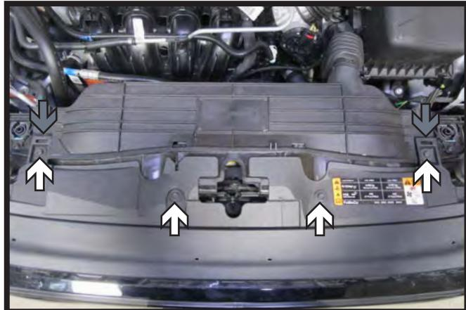
1. Using a 10MM socket, remove the four (4) bolts (white) from the top edge of the fascia. There are two (2) on each side. Then unclip the two (2) push pins (gray), one (1) on each side.
