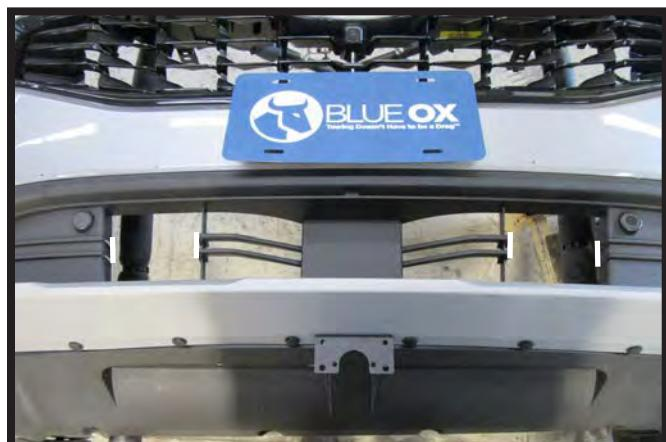
24. Remove the two (2) horizontal slats between the white marks as shown to allow room for the removable tabs and convenience links.
