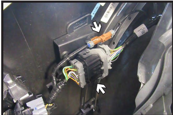
7. Disconnect the two (2) electrical connections on the passenger side of the vehicle. Remove fascia and set aside to be reinstalled later.
