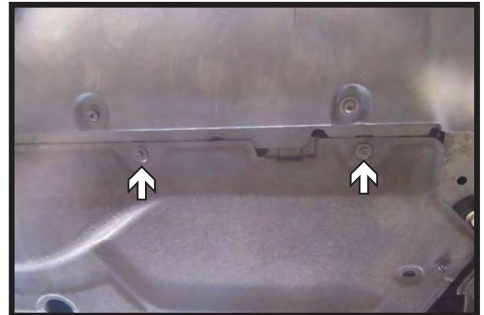
6. Using a 7MM socket, remove the four (4) bolts from the underside of the fascia.
