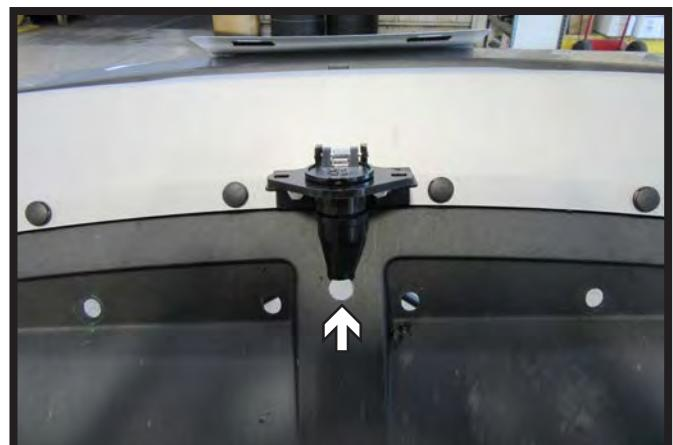
21. Center electrical bracket on bottom of the fascia. Using a 1/4" drill bit, drill two (2) holes using the bracket as a template. Install provided two (2) 1/4" bolts with hardware (left). Hold electrical plug in place and mark fascia below end of plug. Using a 5/8" drill bit, drill one (1) hole to feed tail light electrical wires through (right).
