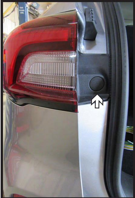
1. Remove the bolt cover from the tail light housing. Do this on both sides of the vehicle.
