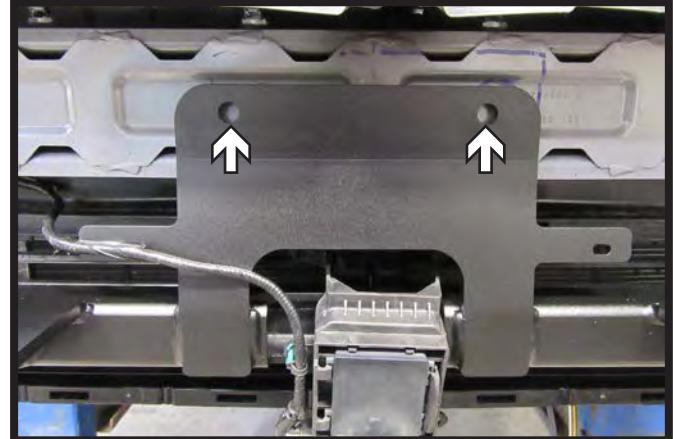
13. Using a 1/2" drill bit, drill out the two (2) holes as shown using the baseplate as a template.
