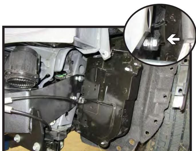
23. Reinstall the black box onto the driver side of the vehicle. Reattach the wire loom to the bottom bolt on the backside. If the box touches the baseplate bolt head, bend back plate slightly to create clearance (inset).
