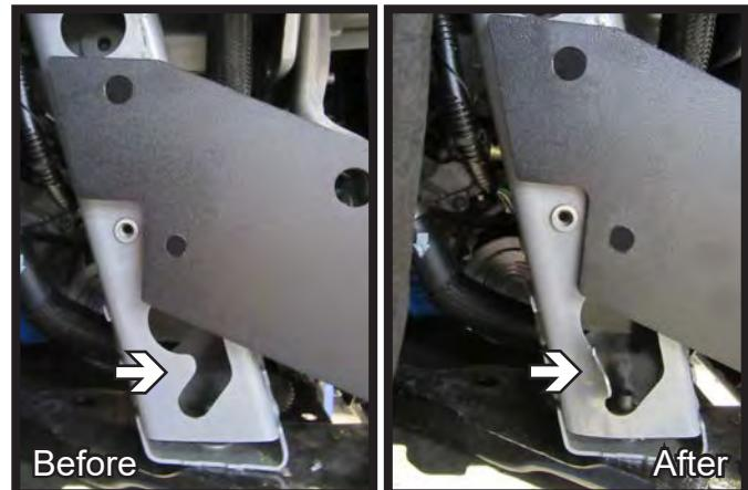
17. Using a pair of large vise grips bend back the frame piece as shown to create an access hole for the nut plate. Do this on both sides of the vehicle.
