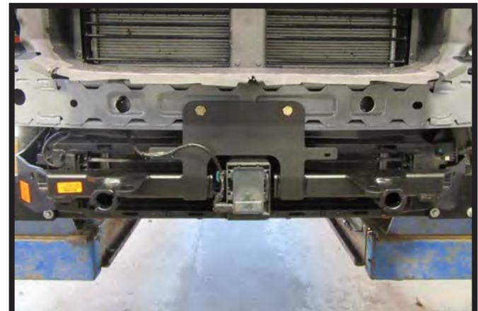
19. Reinstall the four (4) bolts attaching the ACC to the frame.
