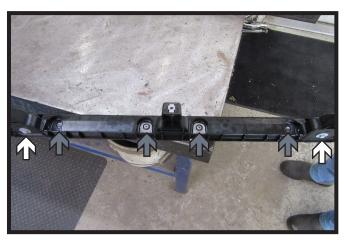
10. Using a 10MM socket, remove the two (2) bolts (white) from the plastic piece on the bottom of the bumper. Then using a 1/4" drill bit, drill out the four (4) plastic rivets (gray). Remove plastic piece and set aside to be reinstalled with the baseplate.
