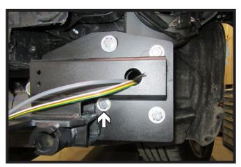
15. Install one (1) 1/2" x 1-1/2" bolt with flat washer and nylon lock nuts into the bottom inside hole on the front of the baseplate. Leave loose at this time. Do this on both sides of the vehicle.
