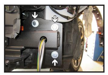
11. Hold baseplate in place and start the three (3) 1/2" x 1-1/2" bolts with flat washers and nylon lock nuts. Snug up the baseplate into place but leave loose. Do this on both sides of the vehicle.
