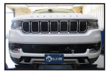
19. Hold the fascia as close to its original position, mark and trim the fascia around electrical rods. Reinstall the fascia and reconnect all electrical connections.
