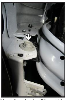
3. Pull back the wheel well liner. Using a 10MM socket, remove the one (1) bolt from the fascia joint. Do this on both sides of the vehicle.
