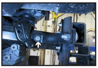
14. Install one (1) 1/2" bolt with lock washer and whiz nut. Do this on both sides of the vehicle.
