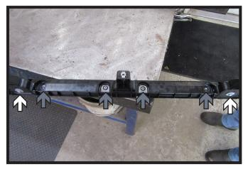
Using a 10MM socket, remove the two (2) bolts (white) from the plastic piece on the bottom of the bumper. Then using a 1/4" drill bit, drill out the four (4) plastic rivets (gray). Remove plastic piece and set aside to be reinstalled with the baseplate.
