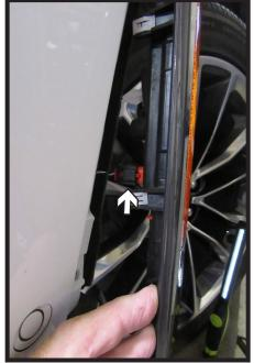
Unsnap the wheel well trim past the fascia joint. Unplug light as trim is pulled back. Place soft cloth between trim and vehicle to hold trim out of the way. Do this on both sides of the vehicle.
