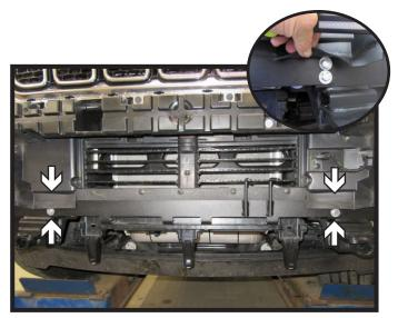
Pull back plastic shroud (inset) and attach cross member to baseplates, start the four (4) 3/8" x 1-1/4" bolts with flat washers and nylon lock nuts. Ensure baseplate is level and tighten baseplate on each side then cross member.
