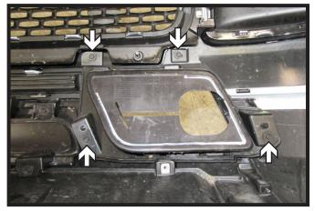
Using a 7MM socket, remove the four (4) bolts from the plastic piece on the back of the fascia. Remove plastic piece and set aside, it will not be reinstalled. Do this on both sides of the vehicle.
