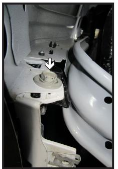
3. Pull back the wheel well liner. Using a 10MM socket, remove the one (1) bolt from the fascia joint. Do this on both sides of the vehicle.
