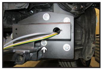
15. Install one (1) 1/2" x 1-1/2" bolt with flat washer and nylon lock nuts into the bottom inside hole on the front of the baseplate. Leave loose at this time. Do this on both sides of the vehicle.
