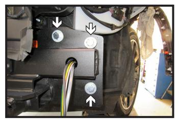
Hold baseplate in place and start the three (3) 1/2" x 1-1/2" bolts with flat washers and nylon lock nuts. Snug up the baseplate into place but leave loose. Do this on both sides of the vehicle.
