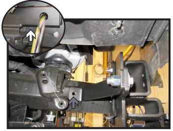
Using a 1/2" drill bit, drill the bottom inside hole on the front of the baseplate (inset). Then using the support bracket as a template, drill 1/2" hole in frame (white). Do this on both sides of the vehicle.
