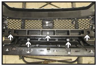
8. Remove the five (5) clips from the foam piece on the back of the fascia. Remove foam piece and set aside, it will not be reinstalled.
