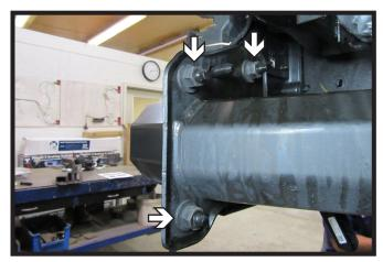
Using an 18MM socket or wrench, remove the three (3) nuts from the bumper. Do this on both sides of the vehicle. Remove bumper, it will not be reinstalled.
