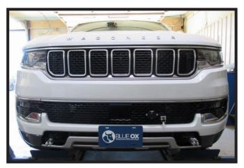
Hold the fascia as close to its original position, mark and trim the fascia around electrical rods. Reinstall the fascia and reconnect all electrical connections.
