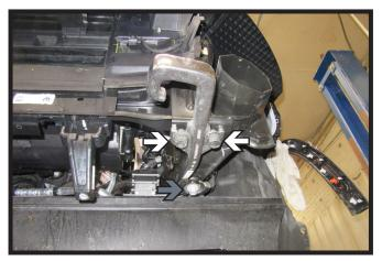
Using a 21MM socket, remove the front two (2) bolts (white) on the tow hooks. Then using an 18MM socket, remove the back one (1) bolt (gray). Remove tow hook, it will not be reinstalled. Reinstall back bolt from tow hook (gray). Do this on both sides of the vehicle.
