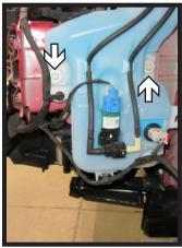
9. On the driver side of the vehicle, using a 10MM socket, remove the one (1) nut from the top of the windshield washer fluid reservoir. Disconnect all lines. Then using a 10MM socket, remove the two (2) bolts at the bottom of the reservoir. Set aside to be reinstalled later.
