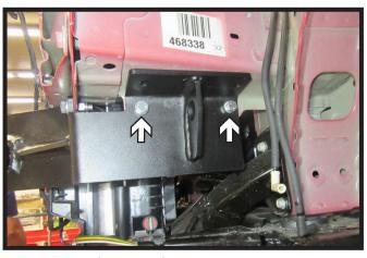
16. Install 3/8" x 1-1/4" bolts with lock washers and lock nuts into bottom two (2) holes. Do this on both sides of the vehicle.
