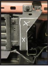
11. Using a utility knife, trim the shutter housing as shown on each side of the vehicle.
