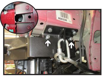
17. Install 3/8" x 1-1/4" bolts with lock washers and nuts plates into top two (2) holes using access hole on front of vehicle (inset). Do this on both sides of the vehicle.
