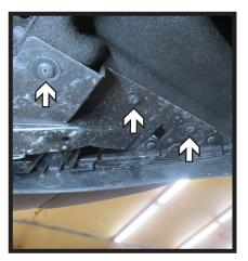
6. Using a T15 Torx, remove the ten (10) bolts from the underside of the fascia. There are three (3) on each side and four (4) in the middle.
