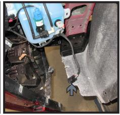
8. Start to remove the fascia. As the fascia is removed unplug the three (3) electrical connections passenger side (white) and one (1) on the driver side (gray) of the vehicle. Remove fascia and set aside to be reinstalled later.
