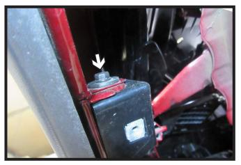
Pull back the wheel well liner. Using a 7MM socket, remove the one (1) bolt from the fascia joint. Do this on both sides of the vehicle.
