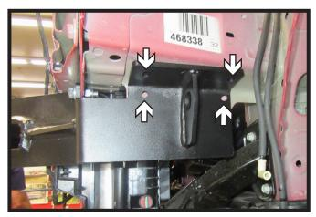
15. Using a 3/8" drill bit, drill the remaining four (4) holes on the side of the vehicle using the baseplate as a template. Do this on both sides of the vehicle.
