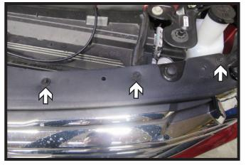
2. Using a 7MM socket, remove the six (6) bolts, three (3) on each side, from the top of the fascia.
