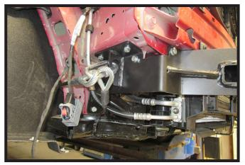
18. Attach the permanent baseplate safety cables to the provided convenience link on the baseplate. The photo above shows the recommended installation of the cables to frame of vehicle. Additional options may interfere with suggested mounting; in this case, secure the cables to a solid piece of the frame as described in the General Information sheet. Be sure the safety cables do not rub against any hoses or moving parts. Do this on **BOTH** sides of the vehicle.
