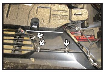
12. Remove the three (3) push pins from the back side of the fascia. Zip tie wire loom straight across below the foam piece.
