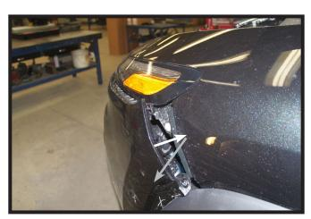
Lift the corners of the fascia up towards 5. the fender (white) and out to release (gray). Continue along under the headlights unsnapping the fascia from the vehicle. Unplug electrical on driver side. Set the fascia aside to be reinstalled later.
