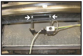
10. Hold electrical/breakaway mounting bracket in place and mark bumper. Using a 1/4" drill bit, drill two (2) holes for the bracket. Attach bracket to the bumper using the two (2) 1/4" bolts and hardware.
