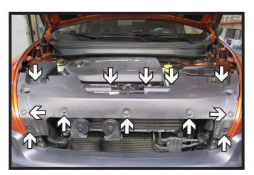
Remove the twelve (12) push pins from the top edge of the fascia cover. There are five (5) on each side and one (1) in the center. Remove fascia cover and set aside to be reinstalled later.
