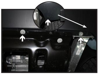
4. Remove the two (2) rivets from the underside corners of the fascia (inset). There is one (1) on each side. Using a 10MM socket, remove the four (4) bolts from the middle portion of the fascia. There are two (2) on each side.
