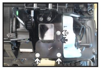
Using a 15MM socket, remove the three (3) bolts (white) from the frame extension. Using a 10MM socket, remove the nut from the fascia extension (gray). Do this on both sides of the vehicle. The extensions will not be reinstalled.
