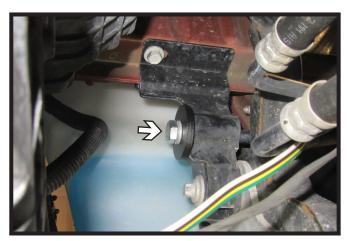
9. From the backside install the 1/2" x 5" bolt with lock washer and 1/4" x 2" DIA washer plate. Do this on both sides of the vehicle.
