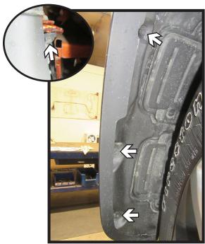
3. Using a 8MM socket, remove the three (3) bolts from the edge of the wheel well. Pull back the wheel well liner, using a 10MM socket, remove the one (1) bolt behind the trim (inset). Do this on both sides of the vehicle.
