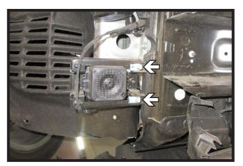
13. Using a 10MM socket, remove the two (2) bolts from the backside of the pedestrian alert system. Remove alert system and set aside to be reinstalled later.
