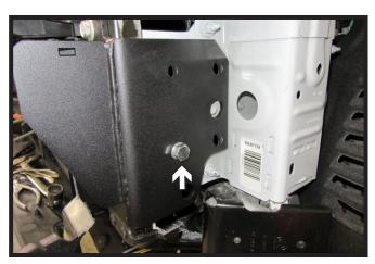
24. Start a 1/2" x 1-1/2" bolt with lock washer and whiz nut in the bottom front hole. Leave loose at this time. Do this on both sides of the vehicle.
