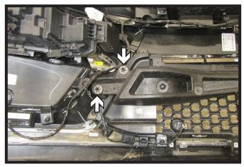
20. On the back side of the fascia, remove the four (4) clips, two (2) on each side, from the foam piece. Remove foam piece, it will not be reinstalled.
