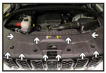
1. Remove the ten (10) push pins from the top of the fascia cover. Remove fascia cover and set aside to be reinstalled later.
