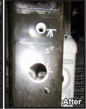
19. Measure 3" from the center of the top hole down. Using a 1-1/4" hole saw, drill hole centering hole with existing holes on the frame and the bottom of the 3" measurement. Do this on both sides of the vehicle as needed.
