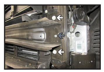
12. Using a 16MM socket, remove the two (2) bolts (white) from the bumper. Then using a 10MM socket, remove the one (1) nut (gray). Do this on both sides of the vehicle. Remove bumper and set aside. It will not be reinstalled later.
