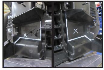
17. Using a utility knife, trim the shroud on each side of the bottom shutters as indicated.
