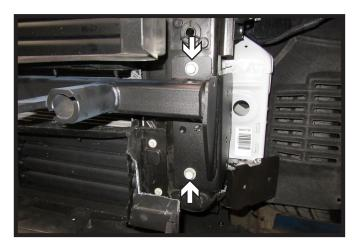
22. Hold baseplate into place on the vehicle frame and start the existing bolts in both front holes. Do this on both sides of the vehicle.
