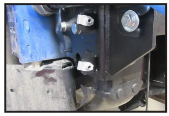
29. Install clips from pedestrian alert bracket onto the tabs on the passenger side of the baseplate.
