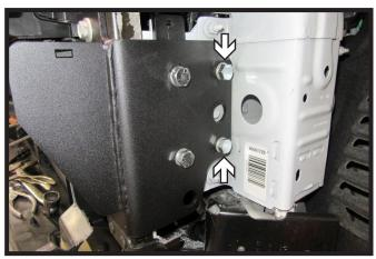
26. Install two (2) 1/2" x 1-1/2" bolts with lock washers and whiz nuts into back holes. Do this on both sides of the vehicle. Tighten all bolts at this time.
