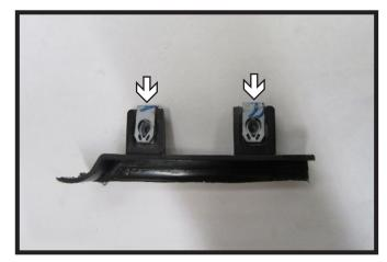
21. Remove clips from the pedestrian alert bracket and set aside to be reinstalled later.
