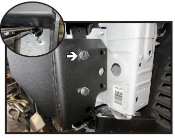
25. Insert spacer plate at top of baseplate between the frame and baseplate with the slotted end facing downward. Once spacer plate is in position insert 1/2" x 1-1/2" bolt with lock washer and whiz nut into top front hole (inset). Leave Loose Do this on both sides of the vehicle.
