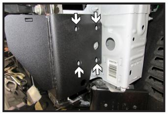
23. Using 1/2" drill bit, drill the four (4) holes on the side of the frame using the baseplate as a template. Do this on both sides of the vehicle.
