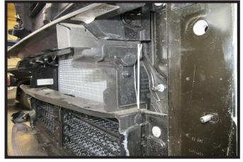
18. Using a utility knife, trim the upper shroud as indicated. Do this on both sides of the vehicle.
