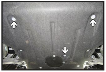
Using a 10MM socket, remove the three (3) bolts from the belly pan. Let belly ban hang.
