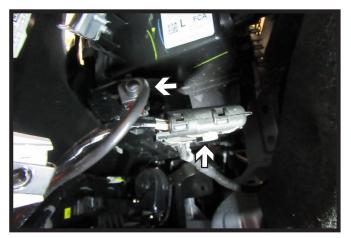
Unplug two (2) electrical connections on the driver side of the vehicle. Remove fascia and set aside to be reinstalled later.
