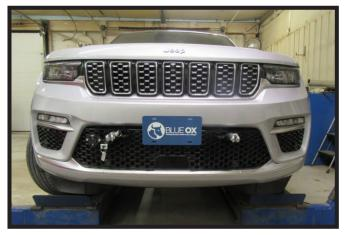
31. Hold the fascia as close to it's original position, mark and trim the fascia around the convenience links and attachment tabs. Reinstall the fascia, fascia cover, and belly pan. Reconnect all electrical connections and windshield washer fluid line.
