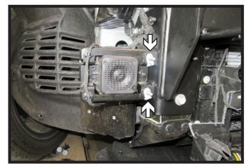
30. Reinstall the pedestrian alert system onto the bracket on the passenger side of the vehicle using the existing bolts and hardware.
