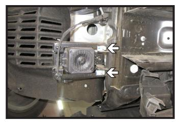
Using a 10MM socket, remove the two (2) bolts from the backside of the pedestrian alert system. Remove alert system and set aside to be reinstalled later.
