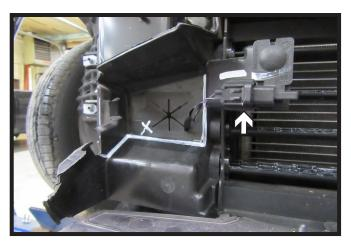
16. Remove the temperature sensor and feed through the plastic on the passenger side of the vehicle. Place out of the way during baseplate installation, it will be reinstalled later.
