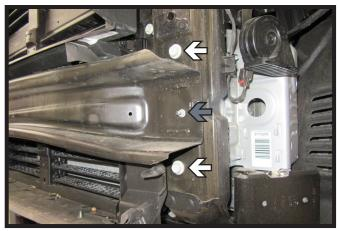
Using a 16MM socket, remove the two
