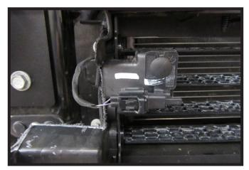
28. Reinstall the temperature sensor on the passenger side of the vehicle. Then reinstall the horns on both sides of the vehicle.
