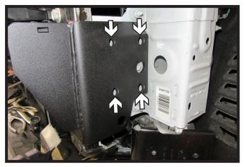
Using 1/2" drill bit, drill the four (4) holes on the side of the frame using the baseplate as a template. Do this on both sides of the vehicle.
