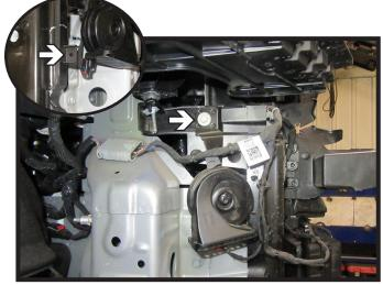
14. Unclip horn from the bracket (inset). Then using a 10MM socket, remove the one (1) bolt. Place the horn out of the way during baseplate installation, it will be reinstalled later. Do this on both sides of the vehicle.
