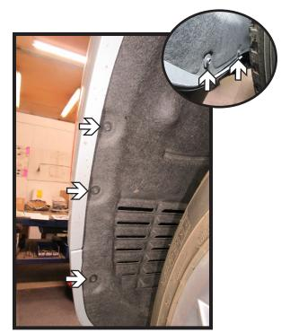
Using an 8MM socket, remove the five (5) bolts from along the edge of wheel well. Do this on both sides of the vehicle.
