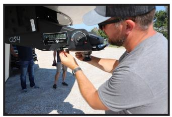
3. Line up the back lockout plate with the carriage bolts and place against the back of the pin box above lip.
