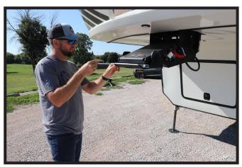
1. Place one (1) of the lockout plates behind the front lip and against the front of the pin box.
