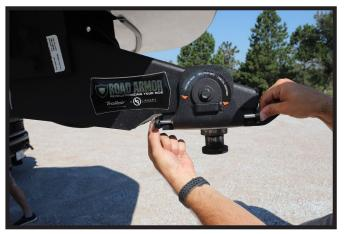
Insert one (1) carriage bolt into each side of the front plate. Feed bolt between pin box and pivot head.
