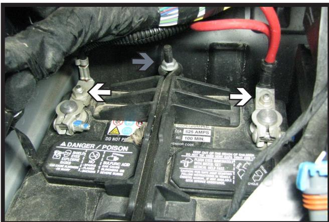
8. On the driver side, using a 10MM socket or wrench, remove the nuts from the battery terminals (white). Using a 13MM socket or wrench, remove the nut from the hold down post (gray). Slide the battery out of the tray and set aside.
