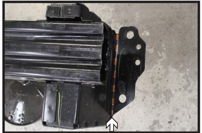
12. Using a reciprocating saw, trim off the outer flanges of the bumper flush with the sides. Do this on both sides of the bumper.
