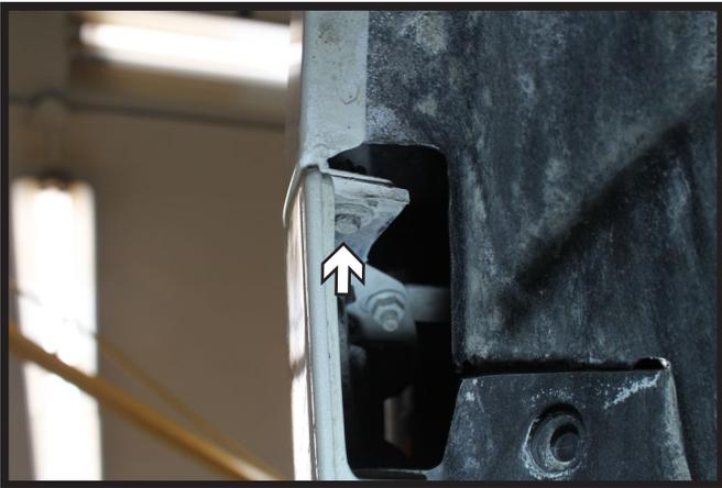
3. Using a 7MM socket, remove the screw from the top edge of the fascia in the wheel well. Do this on both sides of the vehicle.
