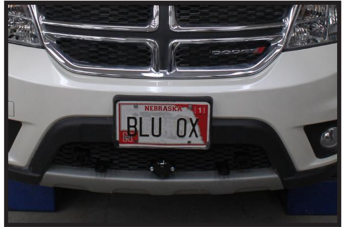
20. Hold the fascia as close to it's original position, mark and trim the lower grille as needed for baseplate clearance. Reinstall the fascia.
