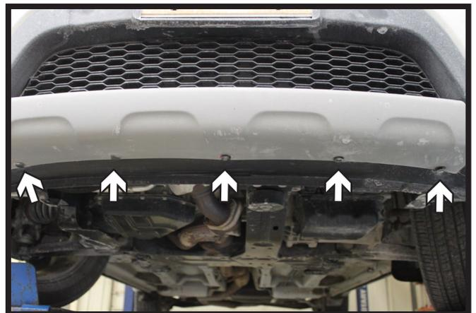
5. Continue along the underside of the fascia removing the five (5) push pins along the front.
