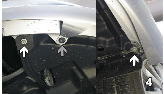
4. Just forward of the front tire underneath, using a 10MM socket, remove the two metric bolts (white arrows). Using a flat screw driver, remove the push pin (gray arrow). Do this on both sides and set aside for later reinstallation.
