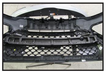
7. Remove the Styrofoam from the back of the fascia by releasing the tabs holding it in place on each side. This will not be reinstalled.
