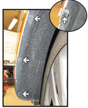
2. Remove the three (3) push pins from along the edge of the wheel well. Using a 10MM socket remove the one bolt (inset). Do this on both sides of the vehicle.
