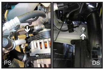
10. Start the two (2) 1/2" bolts with hardware, one (1) on each side, on the inside of the frame as shown. On the driver side this can be accessed from the underside of the vehicle and from above on the passenger side. When tightening the bolt on the passenger side, it is easier to do this from the underside of the vehicle.
