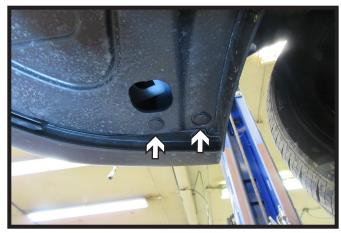
3. Remove the eight (8) push pins from the underside of the fascia. There are four (4) on each side.
