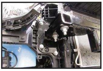
12. Tighten the two (2) 1/2" frame bolts and the eight (8) 8MM bolts on the front of the baseplate. Install the remaining hardware to the four (4) 1/2" cross member bolts and fully tighten.
