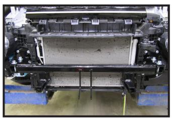
11. Start the remaining four (4) bolts, two (2) on each side to the front of the baseplate. Set the cross tube onto the side brackets. Place the four (4) 1/2" bolts with flat washer and lock washer into holes. Do not add hardware to the bottom of bolts.
