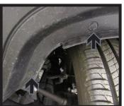
6. Using a 10MM socket, remove the seven (7) bolts (white) from the belly pan. There are four (4) in the front and three (3) in the back. Using a 14MM socket, remove the one (1) plastic bolt (gray) from the belly pan. Then remove the four (4) push pins (black), two (2) from each side. Remove belly pan and set aside to be reinstalled later.
