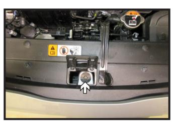
1. Lift the cover next to the handle on top of the fascia. Using a 10MM socket, remove the one (1) bolt.
