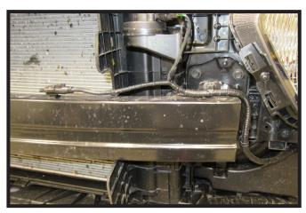
Unclip the temperature sensor wire loom from the bumper on the driver side of the vehicle. Set aside to be reinstalled later.
