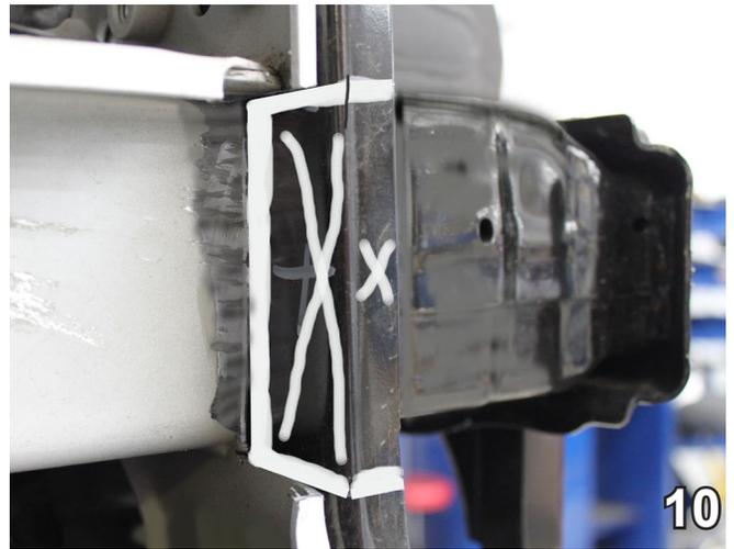
10. Reinstall the front bumper using the existing hardware. Then, use the cut you just made as a template and outline the cut on the back of the front bumper. Use a reciprocating saw and cut this outline out on both sides of the bumper. Reinstall bumper. The radiator cross member will need to be lifted slightly to align holes for bumper reinstallation
