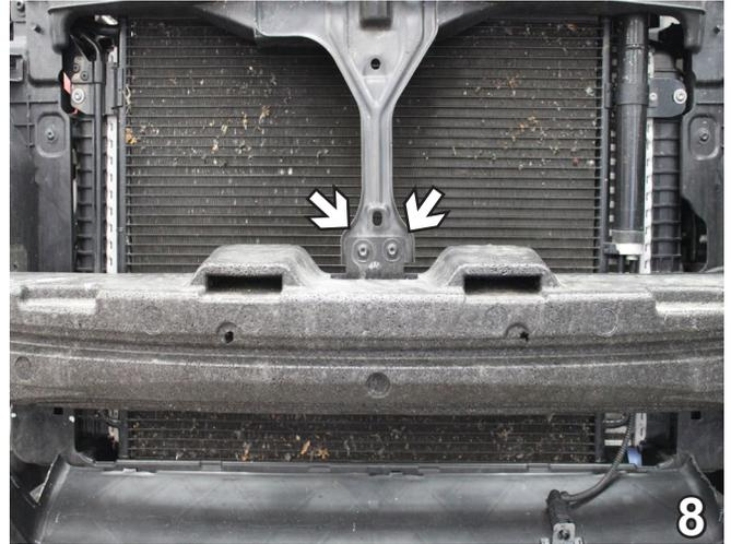
8. Use a T30 Torx to remove the two (2) bolts from the middle of the bumper. Remove the bumper and set bolts and bumper aside to be reinstalled later.
