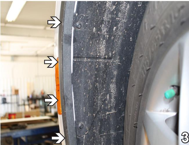
3. Remove the wheel well trim from the driver's side front wheel. To do this, pinch the trim clips from the inside of the wheel well, after pulling back the wheel well. Do this on both sides. Set all parts aside to be reinstalled later.
