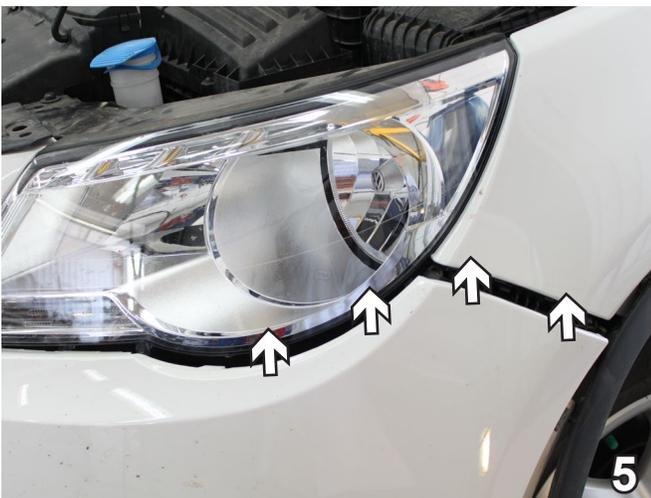
5. To remove the fascia, carefully lift up and out from the vehicle on the edge near the driver's side front wheel. Do this on both sides. Set the fascia aside to be reinstalled later.
