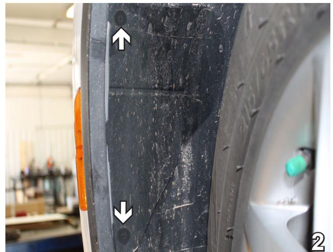
2. In front of the driver's side front tire, use a T30 Torx and remove two (2) bolts from the wheel well. Do this on both sides of the car. Set bolts aside to be reinstalled later.
