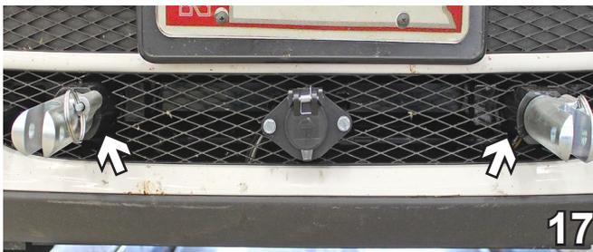
17. Align the fascia to its original position. Trim the grill with a utility knife to allow access to the removable tabs on both sides.
