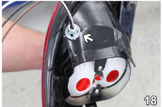
18. Use a 1/2" drill bit, and drill a hole in the back of the tail light. Put the wires through the holes and silicone around it. Reinstall the taillight. Do this on both sides.
