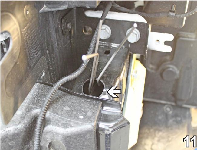
11. Using a 1-1/4" hole saw and a drill, cut downward into the top of the bumper. This hole is to allow nut plates to be placed in later steps. Cut the hole on both sides of the vehicle.
