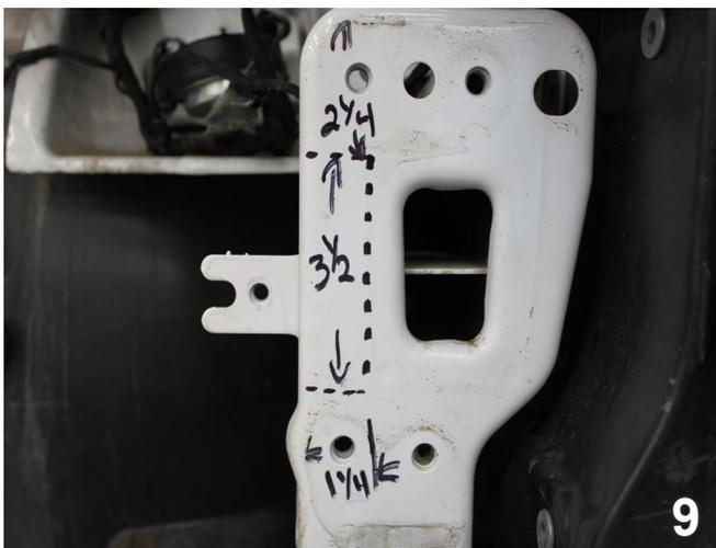
9. Use a reciprocating saw and cut a slot out of the outside of the gray frame webbing on the driver's side. Starting 2-1/4" down from the top of the frame, but in 1-1/4" and down 4-1/2" to allow the baseplate to fit. Do this on both sides.
