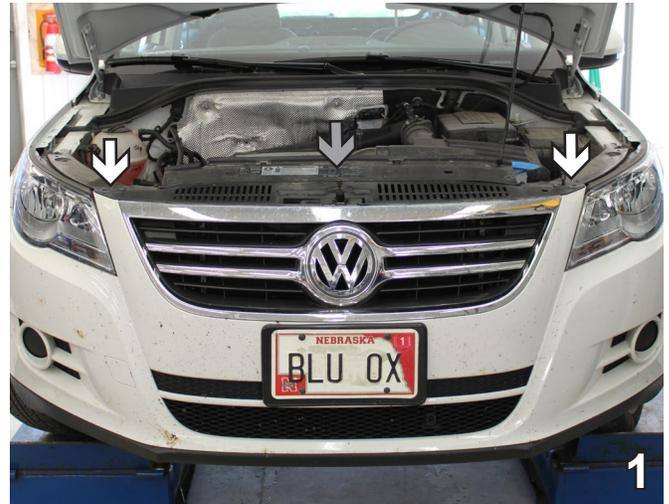
1. Using a T30 Torx, remove the a bolt from each side of the top of the fascia, near each headlight (white arrows). Use a T25 Torx to remove the bolt from the top of the center of the fascia (gray arrow). Set bolts aside to be reinstalled later.
