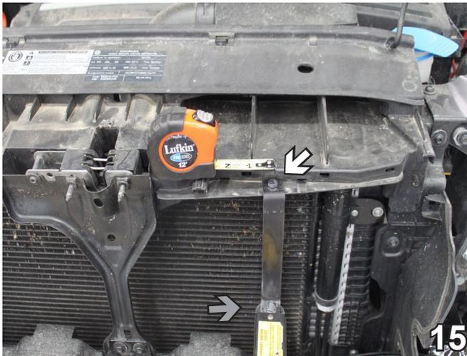
15. **Optional:** To install a breakaway switch use a 1/4" drill bit to make a hole 1" from the driver's side inside fin on the top radiator mounting. Attach the breakaway bracket with a 1/4"-20 x 3/4" hex bolt and a 1/4" hex nylon nut (white arrow). Attach the breakaway switch to the bracket with a 1/4"-20 x 3/4" hex bolt with a 1/4" hex nylon nut (gray arrow). Tighten all bolts with Loctite Red.
