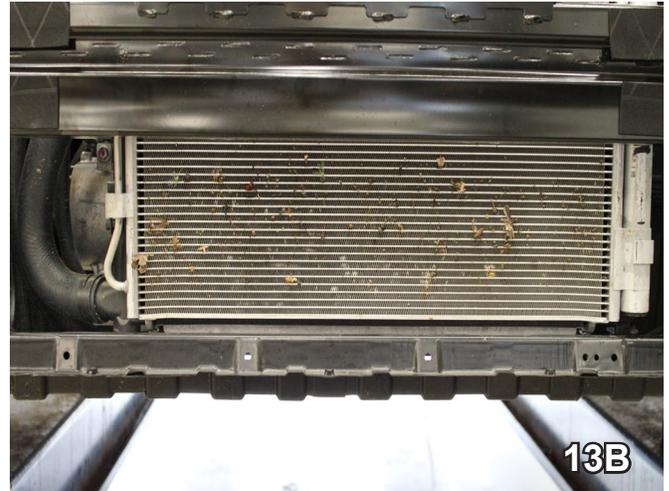
13. On passenger's side only, with utility knife, cut plastic guard even with bottom of metal bumper and remove it from the front of the vehicle (13A). The plastic guard will not be reinstalled. Front view of how the grille looks after plastic guard is removed is shown in 13B.
