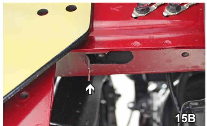
15. Underneath the framerail, with a reciprocating saw, make two (2) horizontal cuts as shown in 15A (between 1" - 1-1/2" long). With a vise grip, bend the metal between the cuts to widen the opening underneath the frame rail (15B). Do this to both sides. These openings will be used to insert the nut plates at a later point in the instructions.
