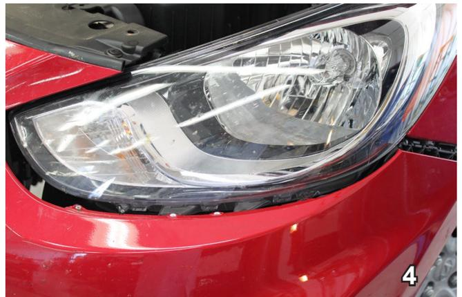
4. To remove fascia, lift up and pull out between the front tire and headlight as shown in the above pictures. Do this to both sides. Set fascia carefully aside to be reinstalled later.
