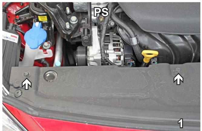
1. To remove radiator cover, with 10MM socket, remove four (4) bolts (white arrows - two (2) per side). To remove additional piece connected to the radiator cover, push in on the push pins and lift up to remove (gray arrows). Set radiator cover in its entirety along with bolts and push pins aside to be reinstalled later.
