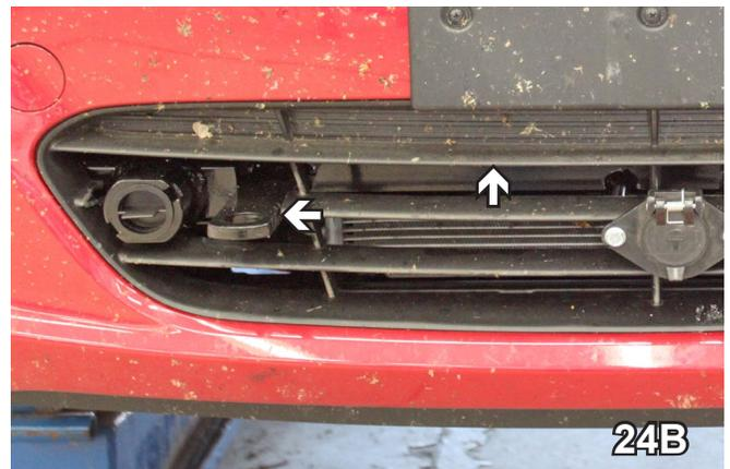
24. In order to accommodate attachment tabs through the fascia of the vehicle, with a utility knife, trim middle piece of fascia referenced in 24A. Do this to both sides of the vehicle. Picture of completed trimming shown in 24B.
