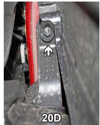
20. Trimming of the air baffle is required before reinstallation. With a utility knife, trim the lower bolt tab off of the air baffle as shown in 20A. A picture of the completed trimming is shown in 20B. Reinstall the air baffle on the driver's side using 6MM-1.00 x 45MM hex bolt with 3/8" flat washer and 3/8" lock washer for top bolt hole (20C) and existing bolt on the bottom side of the air baffle (20D). Tighten bolts with Loctite Red.
