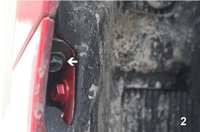
2. In front of tire, with a 10MM socket, remove bolt (white arrow). Do this to both sides. Set bolt aside to be reinstalled later.
