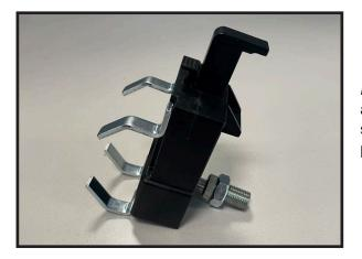
**BRK2521** The BRK2521 brake claw is spring loaded and lockable for safer, faster and easier installs. Simply squeeze the tabs to lock into the open position and push the release button to close.
