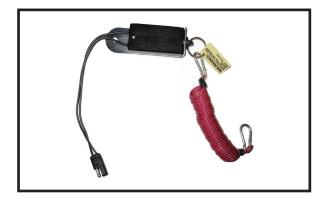
**BRK2505:** There is one (1) breakaway switch included with your Patriot<sup>®</sup>. An additional switch for a second vehicle can be purchased.
