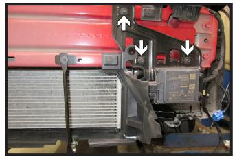
Using a 7MM socket, remove the three
