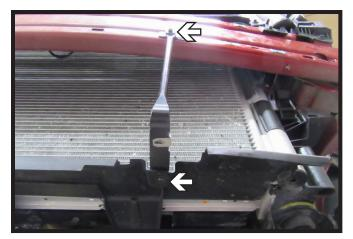
Using a 7MM socket, remove the two (2) bolts from the metal bracket on the front of the vehicle. Do this on both sides of the vehicle. These will be reinstalled later.
