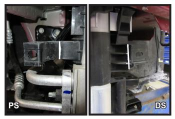
12. Using a reciprocating saw, trim the brackets on the driver and passenger sides of the vehicle as indicated to allow clearance for the baseplate.
