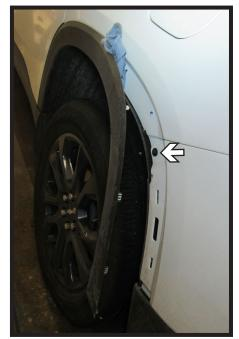
2. Grab the wheel well trim behind the rear tire and pop out the trim past the side and rear panel joint. Keep trim propped away from panels. Then using a 7MM socket remove the one (1) bolt under the trim. Do this on both sides of the vehicle.
