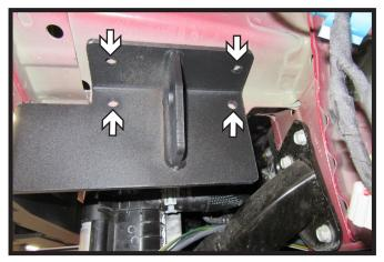
Using a 3/8" drill bit, drill the remaining four (4) holes on the side of the vehicle using the baseplate as a template. Do this on both sides of the vehicle.
