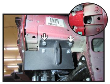
Install 3/8" x 1-1/4" bolts with lock washers and nuts plates into top two (2) holes using access hole on front of vehicle (inset). Do this on both sides of the vehicle.
