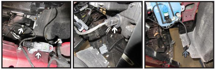
8. Start to remove the fascia. As the fascia is removed unplug the three (3) electrical connections passenger side (white) and one (1) on the driver side (gray) of the vehicle. Remove fascia and set aside to be reinstalled later.
