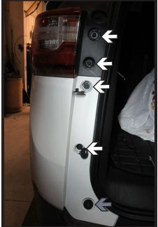
Unpop the covers for the five (5) bolts on the back panel of the vehicle. Then using a 7MM socket, remove the four (4) top bolts (white) and use a T20 Torx to remove the one (1) bottom bolt (gray). Do this on both sides of the vehicle.
