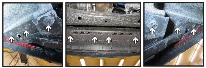
6. Using a T15 Torx, remove the ten (10) bolts from the underside of the fascia. There are three (3) on each side and four (4) in the middle.
