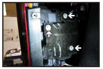
5. Pull back the wheel well liner. Using a 10MM socket, remove the three (3) bolts behind the running lights. Do this on both sides of the vehicle.
