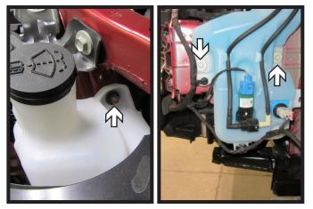
On the driver side of the vehicle, using a 10MM socket, remove the one (1) nut from the top of the windshield washer fluid reservoir. Disconnect all lines. Then using a 10MM socket, remove the two (2) bolts at the bottom of the reservoir. Set aside to be reinstalled later.
