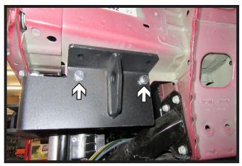
17. Install 3/8" x 1-1/4" bolts with lock washers and lock nuts into bottom two (2) holes. Do this on both sides of the vehicle.
