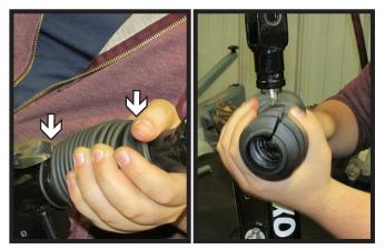
2. Remove the zip ties securing the boot to the leg assembly. Remove the old boot.
