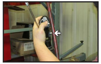
Using a 1/2" socket, remove the one (1) bolt attaching the lug to the leg assembly. Set the lug aside.
