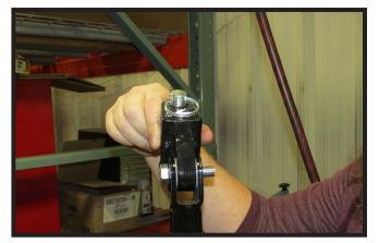
5. Reinstall the lug to the leg assembly.
