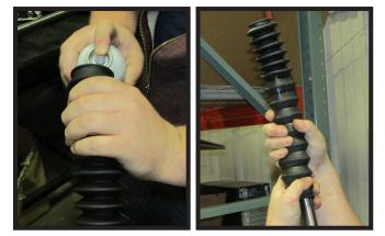
3. Coat the inside of the new boot with silicone spray, clean and re-grease the leg assembly, and install the new boot.
