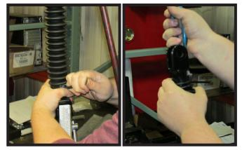
Install the new zip ties onto the boot, ensuring the larger of the two secures the bottom with the smaller on top.
