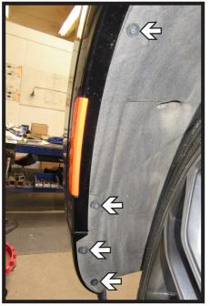
1. Using an 8MM socket, remove the four (4) bolts from the wheel well edge. Do this on both sides of the vehicle.
