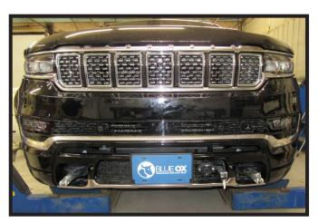
21. Hold the fascia as close to its original position, mark and trim the fascia around electrical rods. Reinstall the fascia and reconnect all electrical connections and hose.
