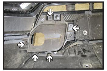
Using a 7MM socket, remove the six
