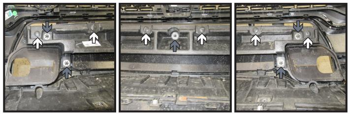
8. Remove the six (6) push pins (white) and five (5) clips (gray) from the foam piece on the back of the fascia. Remove foam piece and set aside, it will not be reinstalled.
