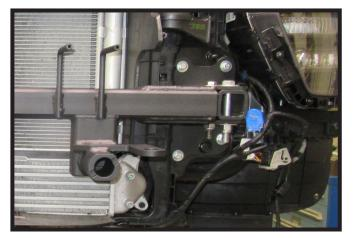
14. Tighten the two (2) 1/2" frame bolts and the eight (8) 8MM bolts on the front of the baseplate. Install the remaining hardware to the four (4) 1/2" cross member bolts and tighten fully.
