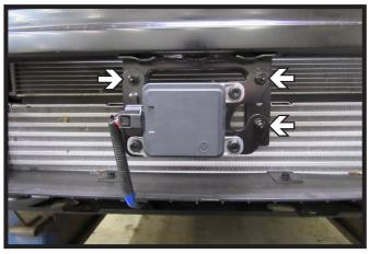
Using a 10MM socket, remove the three
