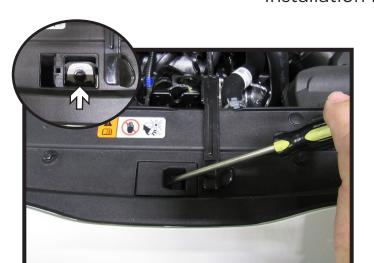
Using a flat screw driver, pop out the plastic piece in the middle of the fascia cover. Using a 10MM socket, remove the one (1) bolt (inset)
