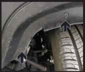
7. Using a 10MM socket, remove the seven (7) bolts (white) from the belly pan. There are four (4) in the front and three (3) in the back. Use your fingers or a 14MM socket to remove the one (1) plastic bolt (gray) from the belly pan. Then remove the four (4) push pins (black), two (2) from each side. Remove belly pan and set aside to be reinstalled later.
