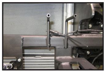
16. Using the provided zip ties attach the temperature sensor loom to the baseplate on the driver side of the vehicle as shown.
