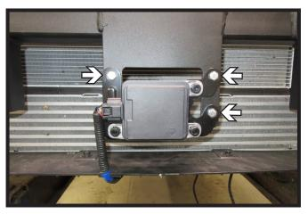
15. Attach the ACC to the bracket on the baseplate using three (3) 1/4" x 3/4" bolts with nylon lock nut.
