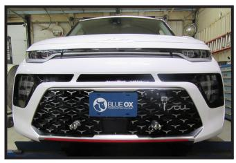
18. Hold the fascia as close to its original position, mark and trim the fascia around the convenience links and attachment tabs. Reinstall the belly pan and fascia.
