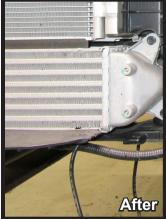
9. Using a reciprocating saw, trim the shroud on each side so that the bottom is flush and the sides are removed as shown.
