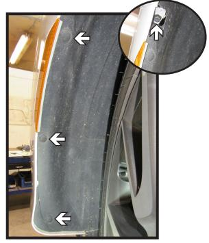
2. Remove the three (3) push pins from along the edge of the wheel well. Using a 10MM socket remove the one (1) bolt (inset). Do this on both sides of the vehicle.
