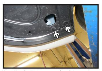
3. Remove the eight (8) push pins from the underside of the fascia. There are four (4) on each side. Remove fascia by lifting and pulling, starting on the side, to release clips along each side as well as the center. Set fascia aside to be reinstalled later.
