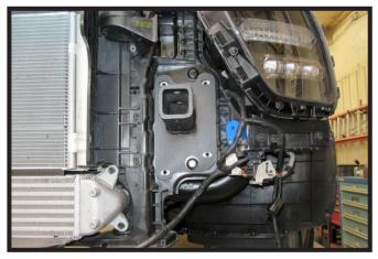
Slide the baseplate into the frame with the hole towards the radiator. Do this on both sides of the vehicle.
