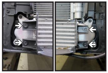
8. Using a 10MM socket, remove the four (4) bolts, two (2) on each side, from the plastic shroud.
