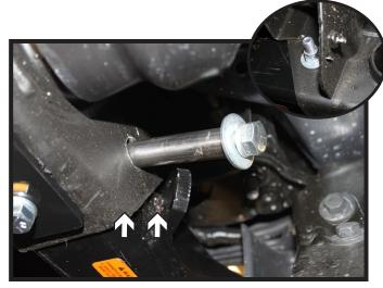
Install the 1/2"-13 x 5" bolt with lock, flat washer and frame sleeve into the inside frame hole. Install a 1/2" flat washer and lock nut onto the bolt on the outside of the frame (inset). Fully tighten all hardware. Do this on both sides of the vehicle.
