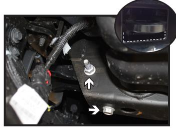
Using a 18MM socket & wrench, remove the two (2) bolts from the tow hook. Remove the tow hook from the vehicle. Do this on both sides of the vehicle.
