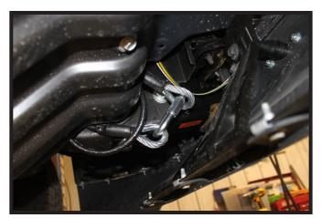
6. Attach the permanent baseplate safety cables to the provided convenience link on the baseplate. The photo above shows the recommended installation of the cables to frame of vehicle. Additional options may interfere with suggested mounting; in this case, secure the cables to a solid piece of the frame as described in the General Information sheet. Be sure the safety cables do not rub against any hoses or moving parts. Do this on **BOTH** sides of the vehicle.
