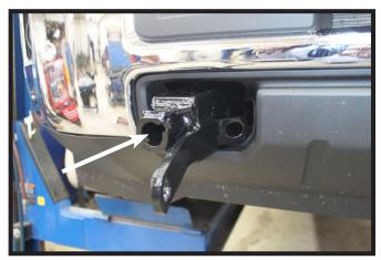
3. Slide the baseplate into the frame thru the tow hook pocket. Do this on both sides of the vehicle.
