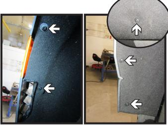
4a. **Tahoe/Suburban Models**: Using a T15 Torx, remove the five (5) screws from the wheel well liner. Do this on both sides of the vehicle.
