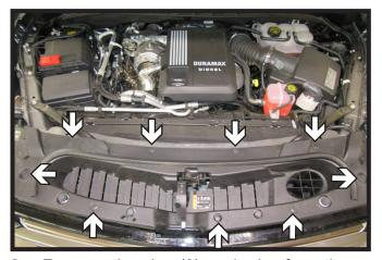
Remove the nine (9) push pins from the fascia cover. Remove facia cover set aside to be re-installed later.
