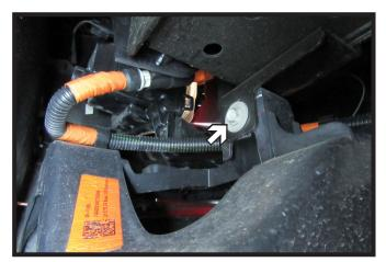
Yukon/Yukon XL Models: Using a 10MM socket, remove the one (1) bolt on the back side of the fascia in front of the tire.
