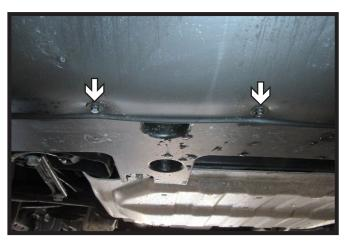
8. Using a 7MM socket, remove the twelve (12) bolts from back of the belly pan, five (5) on each side and two (2) in the middle. Remove belly pan and side covers and set aside to be reinstalled later.
