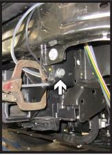
15. Slide the baseplate onto the vehicle and hold in place with vise grips. Install four (4) 1/2" bolts with lock washers and whiz nuts, three (3) bolts on the passenger side and one (1) on the driver side.
