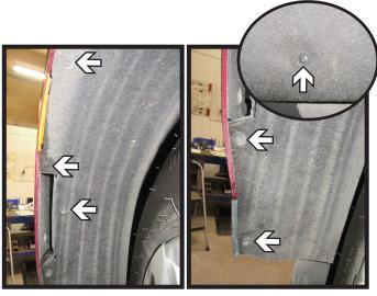
4b. **Yukon/Yukon XL Models**: Using a T15 Torx, remove the six (6) screws from the wheel well liner. Do this on both sides of the vehicle.
