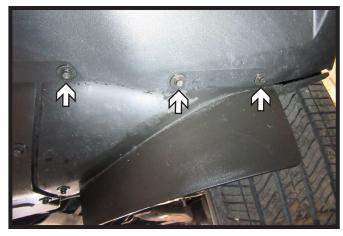
7. Using a 7MM socket, remove the six (6) bolts, three (3) on each side, from the belly pan side covers.
