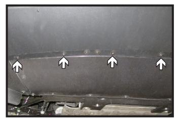
6. Using a T15 Torx, remove the eight (8) screws from belly pan. There are four (4) screws on each side of the vehicle.
