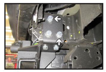
16. Using a 1/2" drill bit, drill the two (2) holes on the driver side using the baseplate as a template. Install the remaining two (2) 1/2" bolts with lock washers and whiz nuts into the side plates.
