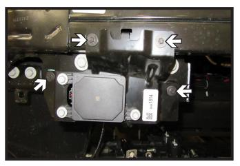
13b. **Models With ACC**: Using a 7MM socket, remove the four (4) mounting bolts from the ACC and allow bracket to hang out of the way. This will be re-installed later. **Note: DO NOT** unplug ACC sensor as it may trip error code on the vehicle.
