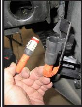
10. Gently pry the fascia loose from the front end. Carefully unplug electrical connections on both sides of the vehicle behind the facia. Remove the fascia from the vehicle and set aside to be reinstalled later.
