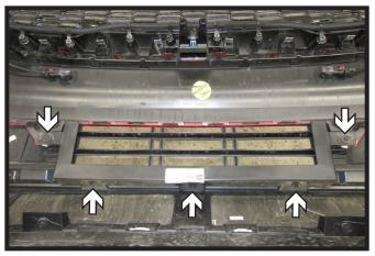
12. **Yukon/Yukon XL Models**: Using a 7MM socket, remove five (5) bolts from plastic piece on back side of fascia. Remove plastic piece, it will not be reinstalled.
