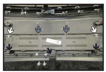
11. **Tahoe Models**: Remove two (2) white clips from cover behind facia (white). Using a T25 Torx, remove two (2) screws from rear cover (gray). Using a 7MM socket, remove the remaining three (3) bolts from the rear cover (black). Remove cover and set aside. This will not be reinstalled.
