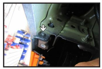
5. Carefully pull back wheel well liner. Using a 7MM socket, remove the one (1) bolt. Do this on both sides.
