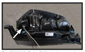
**For BX8869 Only**: Drill a hole according to the tail light wiring kit instructions.
