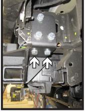
17. Using a 1/2" drill bit, drill the bottom two (2) holes on each side of the vehicle using the baseplate as a template. Then install four (4) 1/2" bolts with lock washers and whiz nuts.
