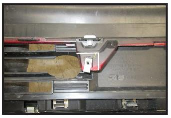
20. Yukon/Yukon XL Models: Trim and remove the indicated area from the back side of fascia to allow clearance for baseplate. Do this on both sides.
