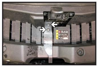
Using a T15 Torx, remove the two (2) screws from the hood latch handle. Remove latch handle and set aside to be re-installed later.
