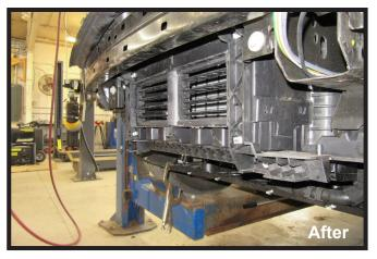
14. Using a reciprocating remove the shutter shroud as shown so that it is flush with the shutter housing.
