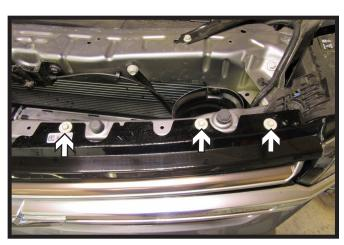
3. Using a 10MM socket, remove the six (6) bolts from top of facia. There are three (3) on each side of the vehicle.
