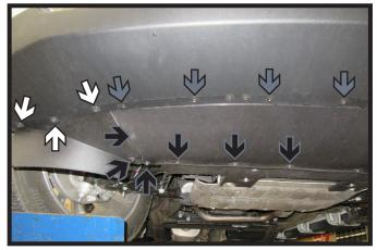
Using a 7MM socket, remove the three (3) bolts from the lower belly pan side cover (white). Do this on both sides. Using a T15 Torx, remove the eight (8) screws from belly pan (gray). Four (4) on each side. Using 7MM socket, remove twelve (12) bolts from belly pan (black), six (6) on each side. Remove belly pan and side covers and set aside to be re-installed later.
