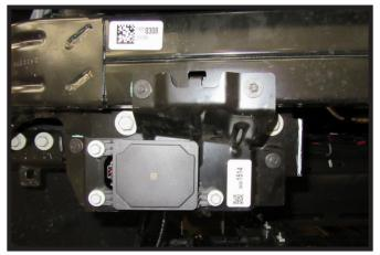
15. Models With ACC: Re-install the ACC bracket.
