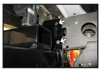
12. On passenger side only, mark the two (2) rear holes on the side of the frame that need to be drilled through. Remove baseplate and set aside. Using a 1/2" drill bit, drill two (2) holes into the side of the frame.
