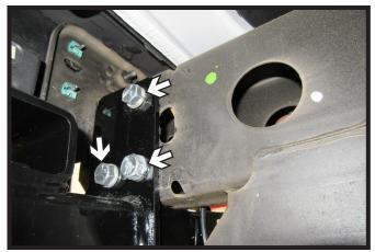
13. Slide baseplate back into place. Using one (1) 1/2" bolt on each side, insert into an existing hole to hold in place. Again, clamp baseplate firmly against bottom of frame on both sides. Install three (3) 1/2" x 1-1/2" bolts with lock washers and wire nuts in the side mounting holes. Tighten fully. Do this on both sides of the vehicle.
