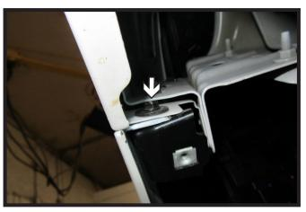
Carefully pull back wheel well liner. Using a 7MM socket, remove the one (1) bolt. Do this on both sides of the vehicle.
