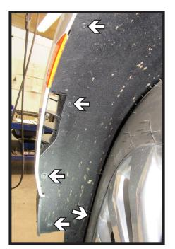
3. Using a T15 Torx, remove the five (5) screws from the wheel well liner. Do this on both sides of the vehicle.
