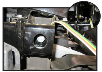
14. Using a 1/2" drill bit and the baseplate holes as a guide, drill the one (1) hole through the bottom of the frame. Do this on both sides. Install 1/2" x 1-1/2" bolt with lock washer and wire nut in bottom mounting hole. Tighten fully. Do this on both sides of the vehicle.
