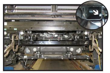
Slide baseplate into place. Using one (1) supplied 1/2" bolt on each side, insert into an existing hole to locate baseplate and hold in place. Using a vise grip, clamp baseplate firmly against bottom of frame on both sides.
