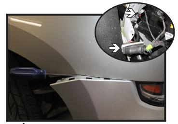
7. A Gently pry the fascia loose from the front end. Carefully unplug two (2) electrical connections on the passenger side behind the facia (inset). Remove the fascia from the vehicle and set aside.
