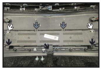
8a. Chevy Tahoe: Remove two (2) white clips from cover behind facia (white). Using a T25 Torx, remove two (2) screws from rear cover (gray). Using a 7MM socket, remove the remaining three (3) bolts from the rear cover (black). Remove cover and set aside. This will not be re-installed.
