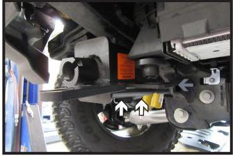
Install baseplate on to frame using the two (2) existing bolts with socket and socket extension. Do this on both sides of the vehicle.
