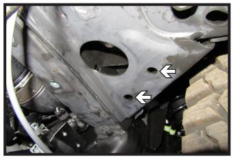
4. Using a 1/2" drill bit, drill out the two (2) holes on the frame next to the tow hook in front of the tire.
