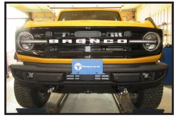
9. Hold skid plate as close to its original position, mark and trim the skid plate around the convenience links and attachment tabs. Reinstall skid plate.
