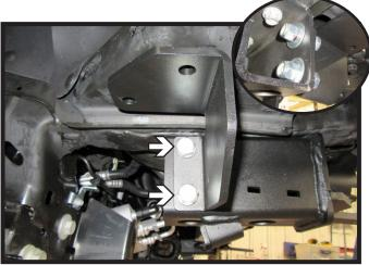
Attached mounting bracket to the baseplate using two (2) 1/2" x 1-1/2" bolts with lock washers and flat washers with nylon lock nuts on the inside of the baseplate tube (inset). Leave bolts loose at this time. Do this on both sides of the vehicle.
