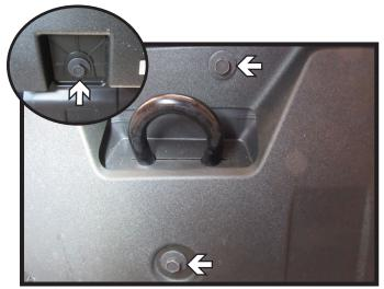
Using a 15MM socket, remove the three (3) bolts from the skid plate. Do this on both side of the vehicle. Remove skid plate and set aside to be reinstalled later.
