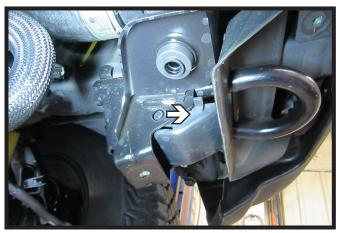
2. Pinch back area of plastic shroud and remove from tow hook. Do this on both sides of the vehicle.
