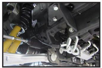
8. Attach the permanent baseplate safety cables to the provided convenience link on the baseplate. The photo above shows the recommended installation of the cables to frame of vehicle. Additional options may interfere with suggested mounting; in this case, secure the cables to a solid piece of the frame as described in the General Information sheet. Be sure the safety cables do not rub against any hoses or moving parts. Do this on **BOTH** sides of the vehicle.
