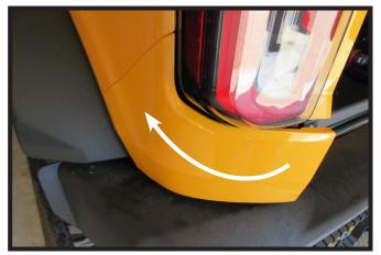
3. Carefully unsnap and remove plastic piece below tail light. Do this on both sides of the vehicle.
