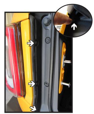
Using a Phillip's screw driver, remove the four (4) push pins. There are three (3) along the edge and one (1) at the top (inset). Unsnap black plastic piece and set aside to be reinstalled later. Do this on both sides of the vehicle.
