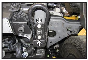
3. Using a 15MM socket, remove the two (2) bolts attaching the tow hook/housing to the frame. Remove tow hook/housing and set aside, it will not be reinstalled. Do this on both sides of the vehicle.
