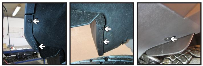
2. Using a T15 Torx, remove the five (5) screws from in front of the tire in the wheel well. Do this on both sides of the vehicle.
