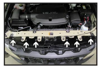
2. Using a T15 Torx, remove the six (6) bolts from the top edge of the fascia.
