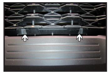
7. Using a 10MM socket, remove the two (2) bolts from the grille.
