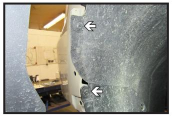
5. Using a T15 Torx, remove two (2) bolts from the wheel well liner. Do this on both sides of the vehicle.
