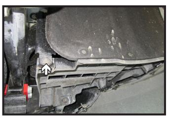
5. Using a 7MM socket, remove the one (1) bolt in front of the tire. Do this on both sides of the vehicle.
