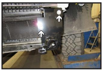
4. Start the two (2) existing 10MM bolts into the front holes. May need to lift baseplate for holes to line up. Tighten bolts but do not use Loctite Red at this time. Do this on both sides of the vehicle.
