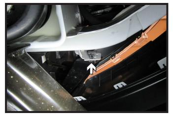
7. Using a flat blade screwdriver unsnap the two (2) clips open on the back side of the fascia. Do this on both sides of the vehicle. Remove fascia and set aside to be reinstalled later.
