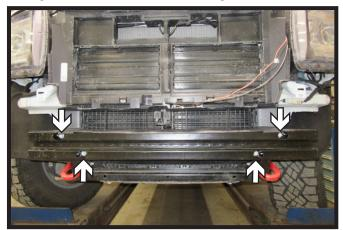
Using a 15MM socket, remove the four (4) bolts from the bumper. There are two (2) bolts on each side of the vehicle. Remove bumper and set aside to be reinstalled later.
