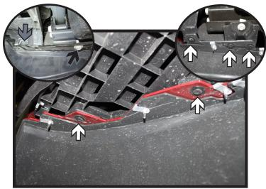
5. **All Models**: Using a T15 Torx, remove the ten (10) screws from the underside edge of the fascia. There are five (5) on each side (white).
