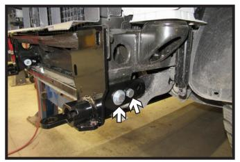
Slide baseplate into place and insert two (2) 1/2" x 3-1/2" bolts into the side holes. Use a flat washer with front bolt. Do not install nuts at this time. Do this on both sides of the vehicle.
