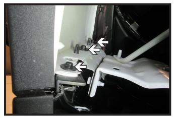
Behind the wheel well liner, using a 7MM socket, remove the three (3) screws along the fascia/fender joint. Do this on both sides of the vehicle.
