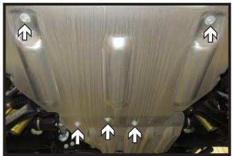
Using a 15MM socket, remove the five (5) bolts from the skid plate. There are two (2) bolts towards the front and three (3) towards the back. Remove skid plate and set aside to be reinstalled later.
