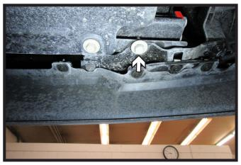
Using a 15MM socket, remove the one (1) bolt from the underside of the fascia. Do this on both sides of the vehicle. Remove fascia and set aside to be reinstalled later.
