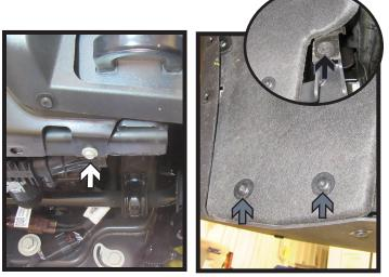
Using a 10MM socket, remove the one
