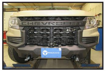
8b. Reinstall the fascia and skid plate. **Note:** May need to trim around tabs and convenience links for proper fit.
