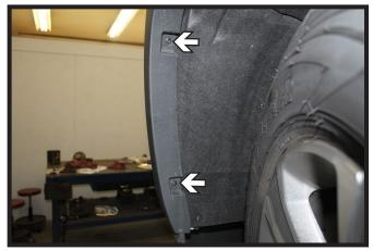
Using a T15 Torx, remove the four (4) screws from the edge of the fender flare. Do this on both sides of the vehicle.
