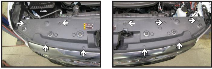
1. Remove the nine (9) push pins from the fascia cover. Remove fascia cover and set aside to be reinstalled later.
