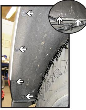
4. Using a T15 Torx, remove the six (6) bolts from along the edge of the wheel well. Do this on both sides of the vehicle.
