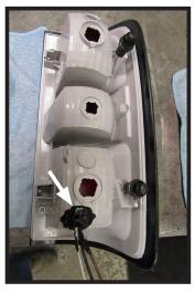
Drill a hole according to the tail light wiring kit instructions.
