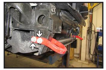
Using an 18MM socket and wrench, remove the two (2) bolts from the tow hook. Do this on both sides of the vehicle. Remove the tow hooks and set aside. They will not be reinstalled later.
