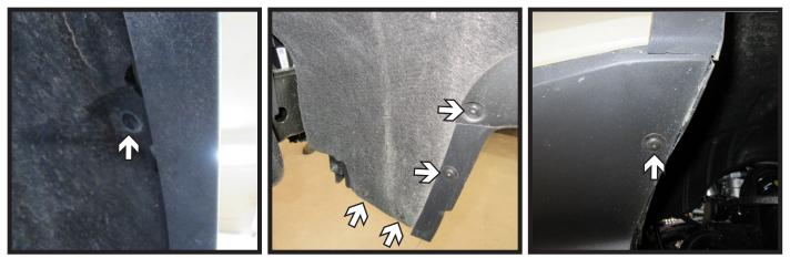
3. Using a T15 Torx, remove the six (6) bolts from along the edge of the wheel well and under the vehicle. Do this on both sides of the vehicle.
