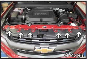
Canyon Only: Remove the nine (9) push pins, four (4) on each side and one (1) in the center, from the fascia cover. Set aside cover to be reinstalled later.
