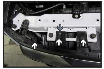
Using a T15 Torx, remove the six (6) bolts (white) and two (2) push pins (gray) from the top edge of the fascia. There are three (3) bolts and one (1) push pin on each side.
