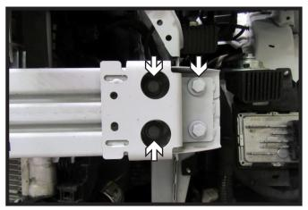
Install the remaining three (3) existing 10MM bolts on each side of the vehicle. Then remove starter bolt from each side and apply Locitie<sup>®</sup> Red and reinstall.
