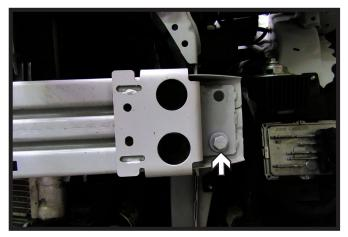
Slide the baseplate between the bumper and the frame. Start one (1) existing bolt on each side of the vehicle to hold baseplate in place.
