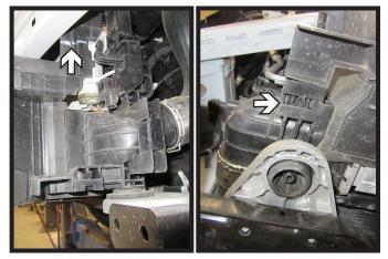
8. Remove the shroud below the bumper by cutting the indicated area (left). Then press clip on bottom of shroud to slide forward and off of the vehicle (right). Do this on both sides of the vehicle.
