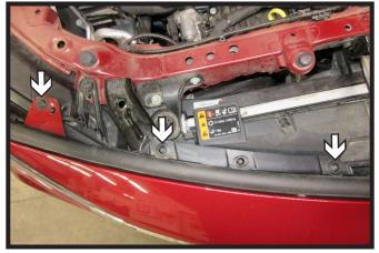
1. Using a T15 Torx, remove the three (3) bolts from the top edge of the fascia. Do this on both sides of the vehicle.
