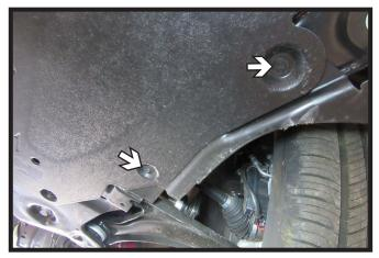
11. Using a 7MM socket, remove the front two (2) bolts on each side of the belly pan. Let belly pan hang.
