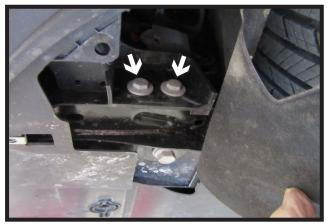
6. Gently pull back lower cover. Using a 13MM socket, remove the two (2) bolts from the underside of the facia. Do this on both sides of the vehicle.
