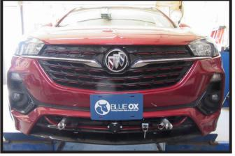
20. Hold the fascia as close to its original position, mark and trim the fascia around the convenience links and attachment tabs. Reinstall the belly pan and fascia.
