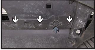
5. Using a 7MM socket, remove the seven (7) bolts (white) from the underside of the fascia. Then remove the two (2) push pins (gray). Unplug electrical connections and remove fascia. Set fascia aside to be reinstalled later.
