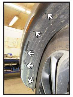
2. Using a T15 Torx, remove the five (5) bolts from along the edge of the wheel well. Do this on both sides of the vehicle.
