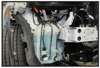
19. Reinstall windshield washer fluid reservoir on passenger side of the vehicle.
