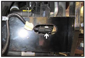
17. Reconnect electrical on passenger side of the vehicle through the hole in the support plate.
