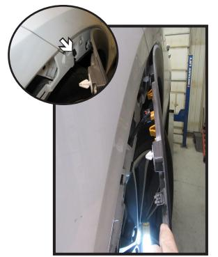
Pull back the wheel well trim and prop away from the vehicle using a soft cloth. Then using a 7MM socket remove the one (1) bolt from the fascia joint (inset). Do this on both sides of the vehicle.
