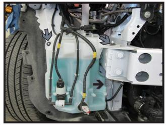
7. Remove the push pin (white) from the top of the windshield washer fluid reservoir on the passenger side of the vehicle. Then using a 10MM socket, remove the two (2) nuts (gray) and one (1) bolt (black) from the reservoir. Plug all lines, remove reservoir, and set aside to be reinstalled later.
