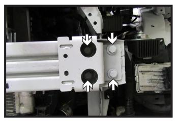
9. Using a 15MM socket, remove the four (4) bolts from the front of the bumper. Do this on both sides of the vehicle. Let bumper hang.
