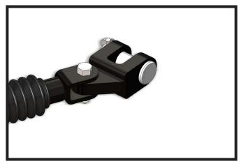
2. Install the offset double lug onto the tow bar leg with the new washers, 1/2"-13 x 2" bolt and 1/2"-13 jam nut provided. Tighten the bolt until the lug is tight against the washers, but can still freely move side to side. Do this on both tow bar legs.
