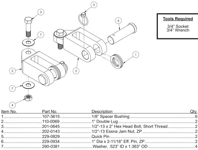
**Note**: If the bumper attachment plate is 5/8"-7/8" thick use the supplied 1/8" bushing(s) between the plate and lug.
