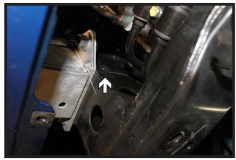
6. Remove the plastic frame plug for nut plate access. Do this on both sides of the vehicle.
