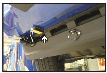
Optional Breakaway: Install the breakaway in the desired location using one of the existing lower outer valance screws.
