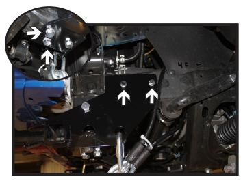
11. Using a 1/2" drill bit, drill the lower existing holes thru the frame. Install the 1/2" hardware and fully tighten both bolts (inset).
