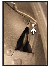
Loosen the wheel well liner by removing the lower screw with a 10MM socket (left) and removing the push pin in the wheel well (right). Pull back the liner to access the frame. Do this on both sides of the vehicle.
