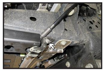
Raptor Models: Reinstall belly pan bracket before installing baseplate safety cables. Do this on both sides of the vehicle.
