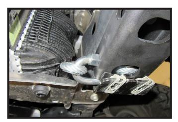
6a. Raptor Models: Attach the permanent baseplate safety cables to the provided convenience link on the baseplate. The photo above shows the recommended installation of the cables to frame of vehicle. Additional options may interfere with suggested mounting; in this case, secure the cables to a solid piece of the frame as described in the General Information sheet. Be sure the safety cables do not rub against any hoses or moving parts. Do this on BOTH sides of the vehicle.
