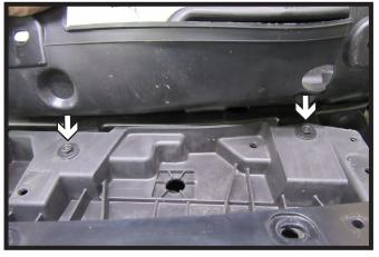
Lift up fascia cover. Using a 10MM socket, remove the two (2) bolts from the top of the fascia. Do this on both sides of the vehicle.
