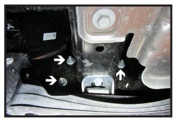
Using a 21MM socket, remove the three
