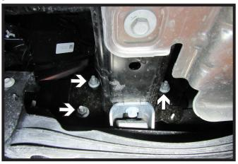
Using a 21MM socket, remove the three
