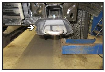
Remove the rubber piece from the tow hook. Do this on both sides of the vehicle.
