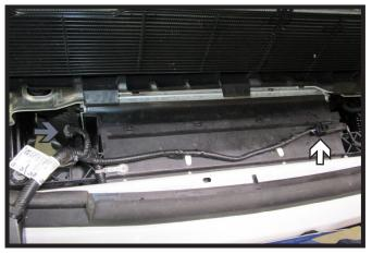
10. Unplug the electrical on the driver side of the vehicle (white), unsnap the wire loom on top of the bumper and then unplug electrical connection on the passenger side of the vehicle (gray). Remove bumper and set aside to be reinstalled later.
