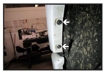
3. Using a 7MM socket or Phillips screw driver, remove the two (2) bolts from along the wheel well edge. Do this on both sides of the vehicle.
