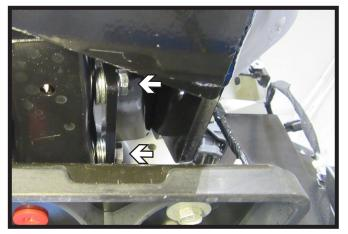
Install the 3/8" hardware into the drilled lower support holes, and fully tighten the bolts, using washers as necessary to ensure tightness.
