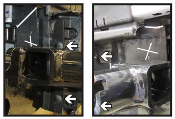
15. Using a reciprocating saw, trim the marked areas on both sides, behind the shutters. Remove two (2) push pins from both sides. (Bottom driver side pin not pictured)
