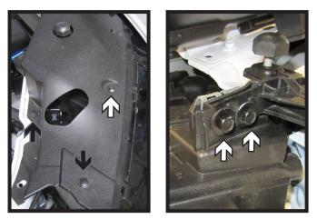
Using a T25 Torx, remove the one (1) screw from the plastic headlight cover (white, left). Remove the two (2) push pins (black). Pull the plastic cover up. Using a 10MM socket, remove the two (2) exposed bolts (white, right). Do this for both sides of the vehicle.
