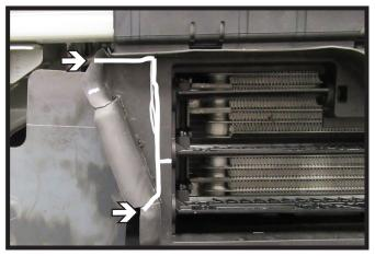
9. Using a reciprocating saw, trim the plastic shielding near the shutters on the passenger side, as shown.
