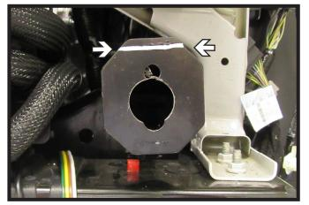
12. Using a reciprocating saw, trim the marked area on the front of the lower support. Do this on both sides of the vehicle.
