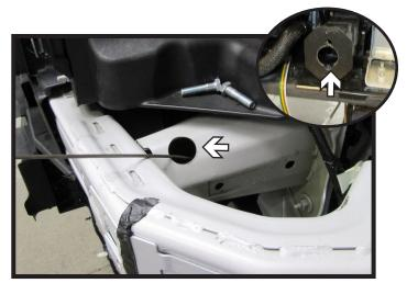
10. Using a 1-1/4" hole saw, drill access holes in the side of the frame as shown and in the face of the lower support (inset). Do this on both sides of the vehicle.
