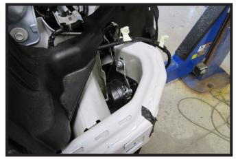
Using a 10MM socket, remove the one (1) bolt from the bumper horn and remove the bracket. Do this for both sides of the vehicle.
