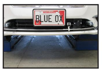
21. Hold the fascia as close to its original position, mark and trim the fascia around the convenience links and attachment tabs. Reinstall the headlights, fascia, and fascia cover.
