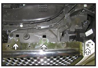
2. Using a 10MM socket, remove the six (6) bolts from the top of the grill cover. There are three (3) on each side.
