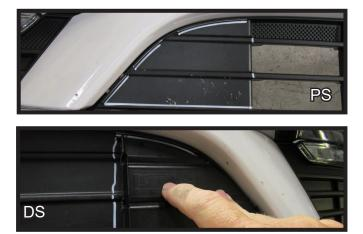
19. Using a reciprocating saw, trim the marked area on the passenger front of the fascia. Use this trimmed piece to mark and cut a similar shape on the driver side.
