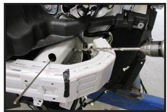
11. Using a 3/8" drill bit, ream out the rear existing hole. Do this on both sides of the vehicle.
