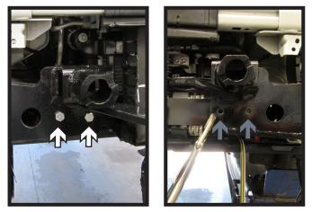
17. Slide the slotted bracket into place and clamp. Install with the supplied 3/8" hardware (white). On the passenger side, using 3/8" drill bit, drill into the bracket (gray). Install with the supplied 3/8" hardware and fully tighten.
