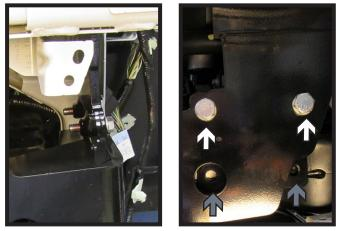
14. Install the lower support plate to the baseplate holes with the supplied 3/8" hardware (white) and fully tighten. Then using a 3/8" drill bit, drill the lower plate holes through the support (gray). Do this on both sides of the vehicle. Fully tighten all hardware.
