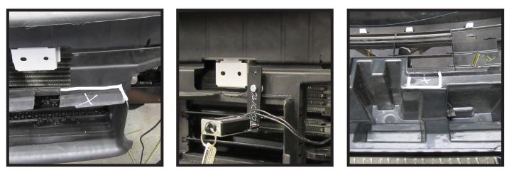
18. **Optional Breakaway:** If installing a breakaway, using a reciprocating saw, cut the marked areas on both the plastic shutter shielding and the fascia. Using a 3/8" drill bit, drill into the baseplate. Install the breakaway with the supplied 3/8" hardware and fully tighten.
