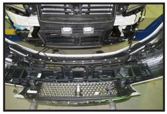
5. Pull the corners of the fascia away from the vehicle disconnecting any electrical connections and set the fascia aside.
