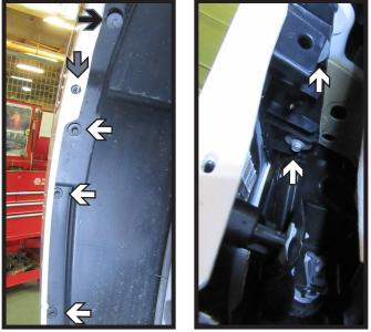
3. Using a 7MM socket, remove the three (3) bolts in front of the tire on the wheel well (white, left). Using a Phillips screwdriver, remove the one (1) screw (gray). Remove the one (1) push pin. Pull the wheel well cover back. Using an 8MM socket, remove the two (2) bolts (white, right). Do this for both sides of the vehicle.
